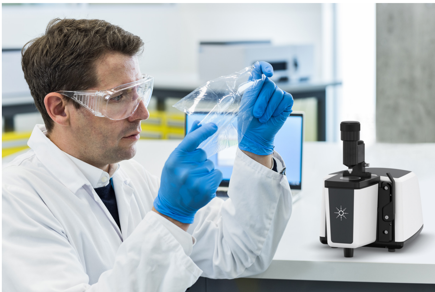
Figure 1. Agilent Cary 630 FTIR spectrometer equipped with an ATR sampling module used for the identification of polymers and thin films.
