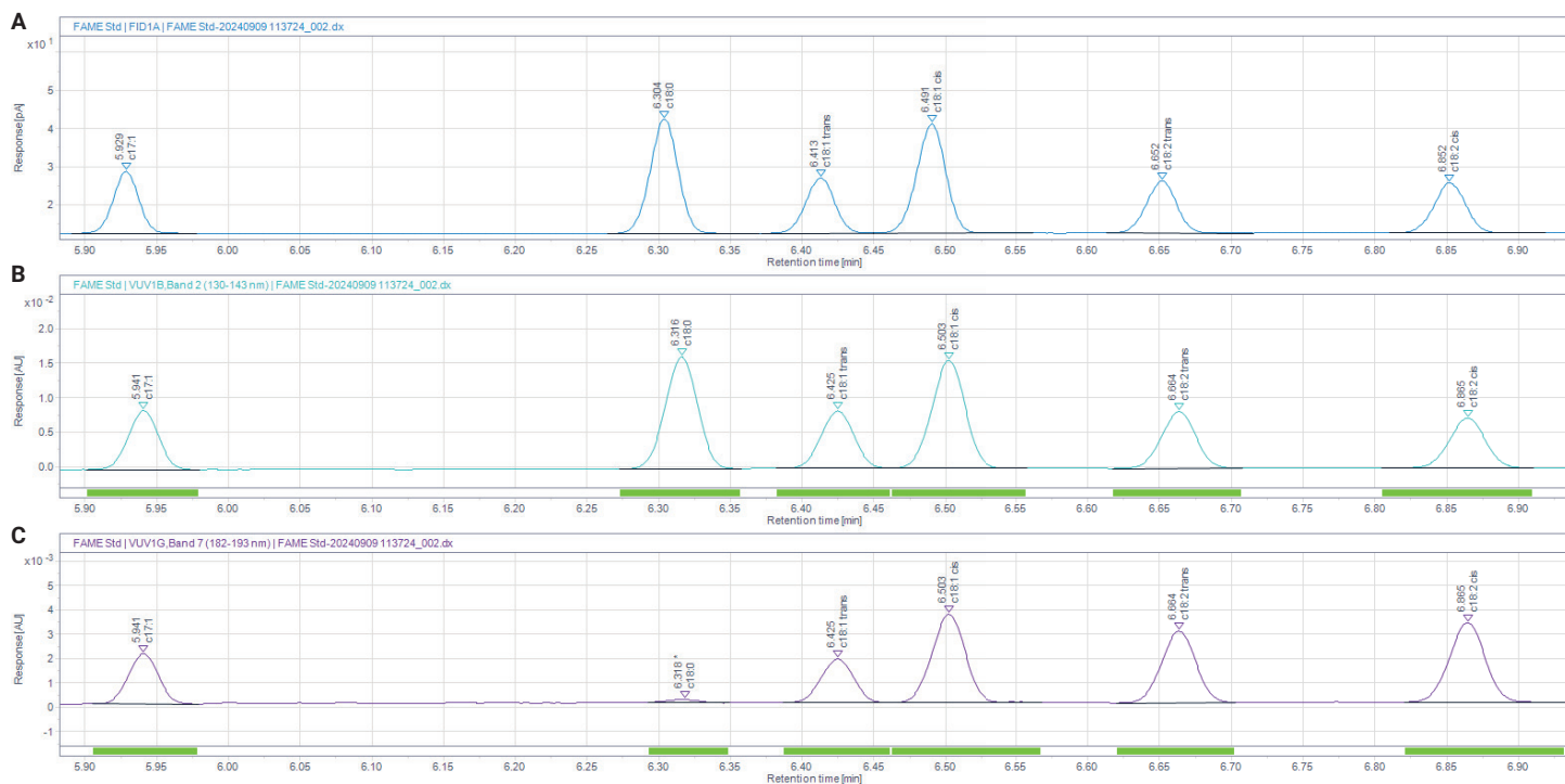
Figure 4. Zoomed-in chromatograms of the c17:1 to c18:3n6 FAMES in the neat standard as analyzed on the FID (A) and LUMA bands 2 (B) and 7 (C).
