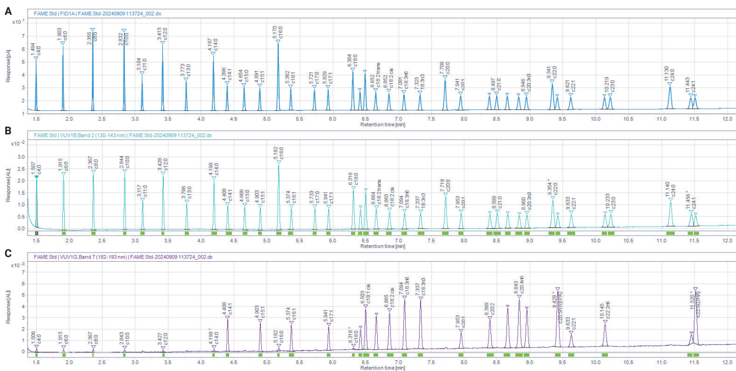
Figure 3. The 37-component FAME mix standard analyzed simultaneously on an FID (A) and LUMA detector bands 2 (B) and 7 (C). UV purity criteria for each peak are highlighted in green or purple in panels B and C.
