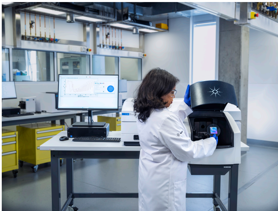
Figure 1. The Agilent Cary 7000 UMS measures absolute reflection and transmission in a single sequence—at variable angle and s or p polarization—without moving or disturbing the sample.
