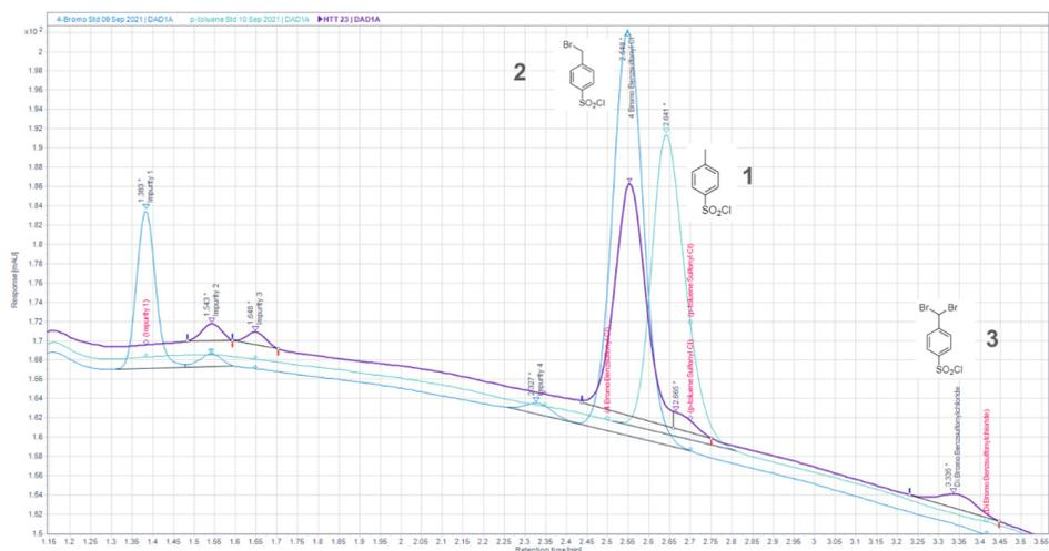
**Figure 3.** Separation of the educt 4-methylbenzenesulfonyl chloride (1, RT = 2.653 min) and the product 4-(bromomethyl)benzenesulfonyl chloride (2, RT = 2.554 min) of the radical bromination reaction. In addition, some impurities (3) and succinimide can be separated. The overlay shows the reaction mixture (purple), educt (turquoise), and product standard (blue).
