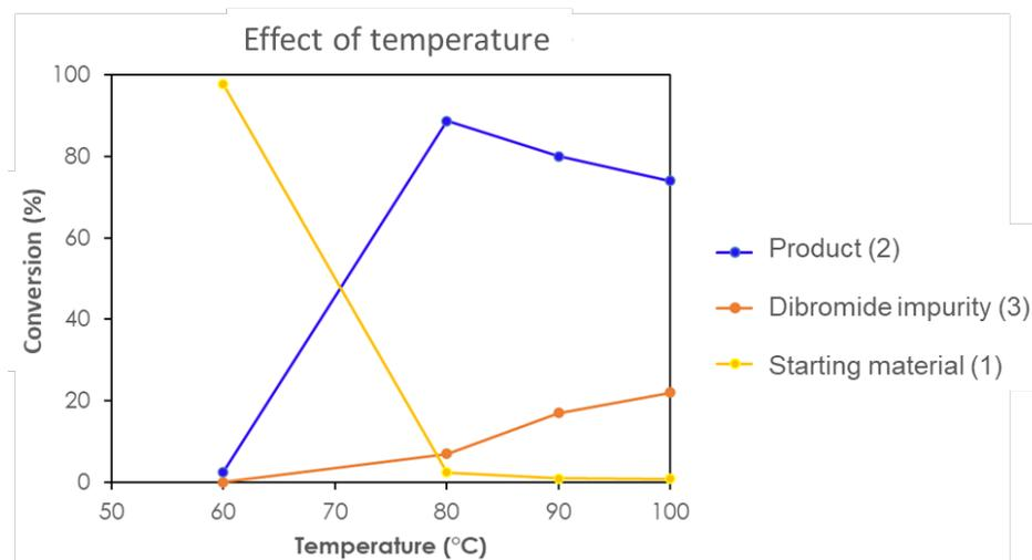
**Figure 5.** Influence of reaction temperature on product yield. Maximum conversion is achieved at 80 °C with the absence of the educt 4-methylbenzenesulfonyl chloride (1). Increasing conversion to the dibromide impurity is observed at temperatures higher than 80 °C. Other reaction conditions include: 0.5 M starting material (1), 0.5 M NBS, 0.047 M AIBN (0.1 eqv.), and 25 min residence time.
