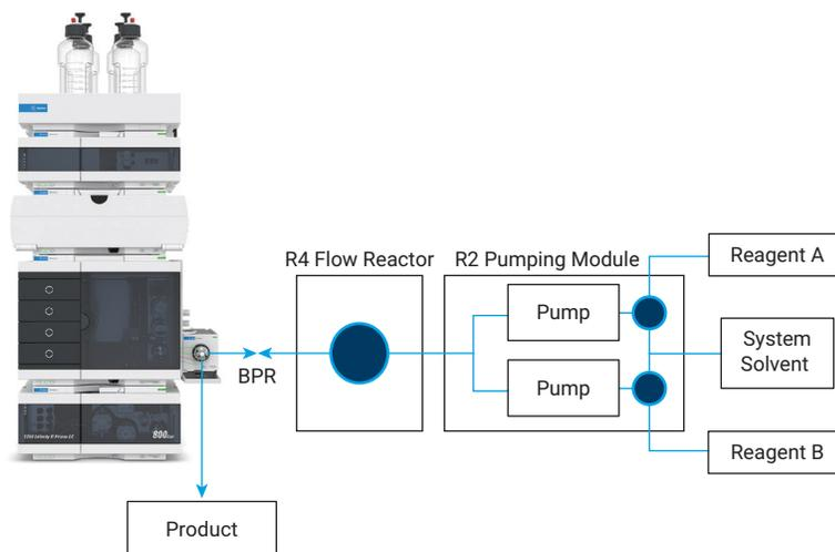
**Figure 2.** Schematic of the Vapourtec R-Series modular flow chemistry system connected to the Agilent InfinityLab Online LC Solution. BPR refers to the backpressure regulator.
