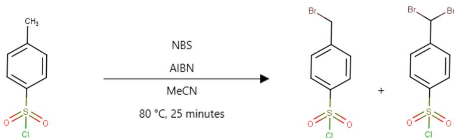
**Figure 1.** Radical bromination of the educt 4-methylbenzenesulfonyl chloride (1) to the product (2) and the dibrominated impurity (3). NBS refers to N-bromosuccinimide, AIBN to 2,2'-azobis(isobutyronitrile), and MeCN to acetonitrile.
