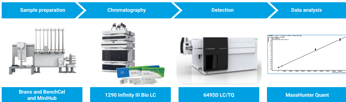
Figure 1. Integrated workflow of the Agilent automated SPE bioanalysis.
