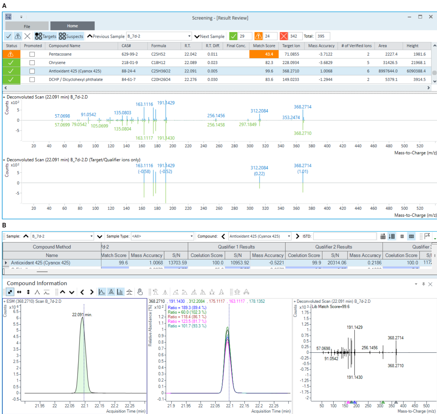
Figure 4. Review of the GC/Q-TOF screener results: (A) Results summary window; (B) Detailed quant batch table.
