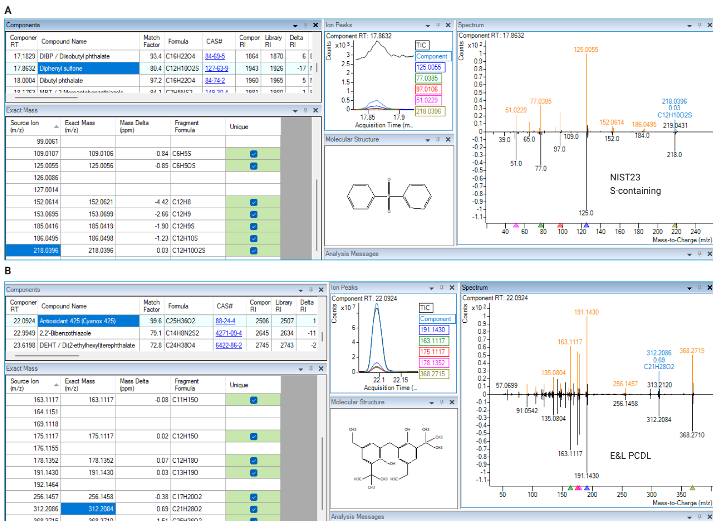
Figure 6. Examples of GC/Q-TOF nontargeted analysis from catheter B using NIST23 library (A) and E&L PCDL (B).
