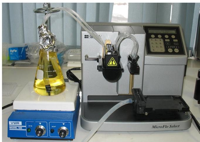
**Figure 1.** Instrument configuration. An Agilent BioTek MicroFlo Select configured with a 10  $\mu$ L tubing cassette.
