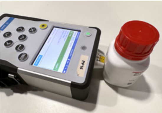
Figure 24. The Agilent Vaya Raman system being used to identify Fmoc-protected amino acids.
