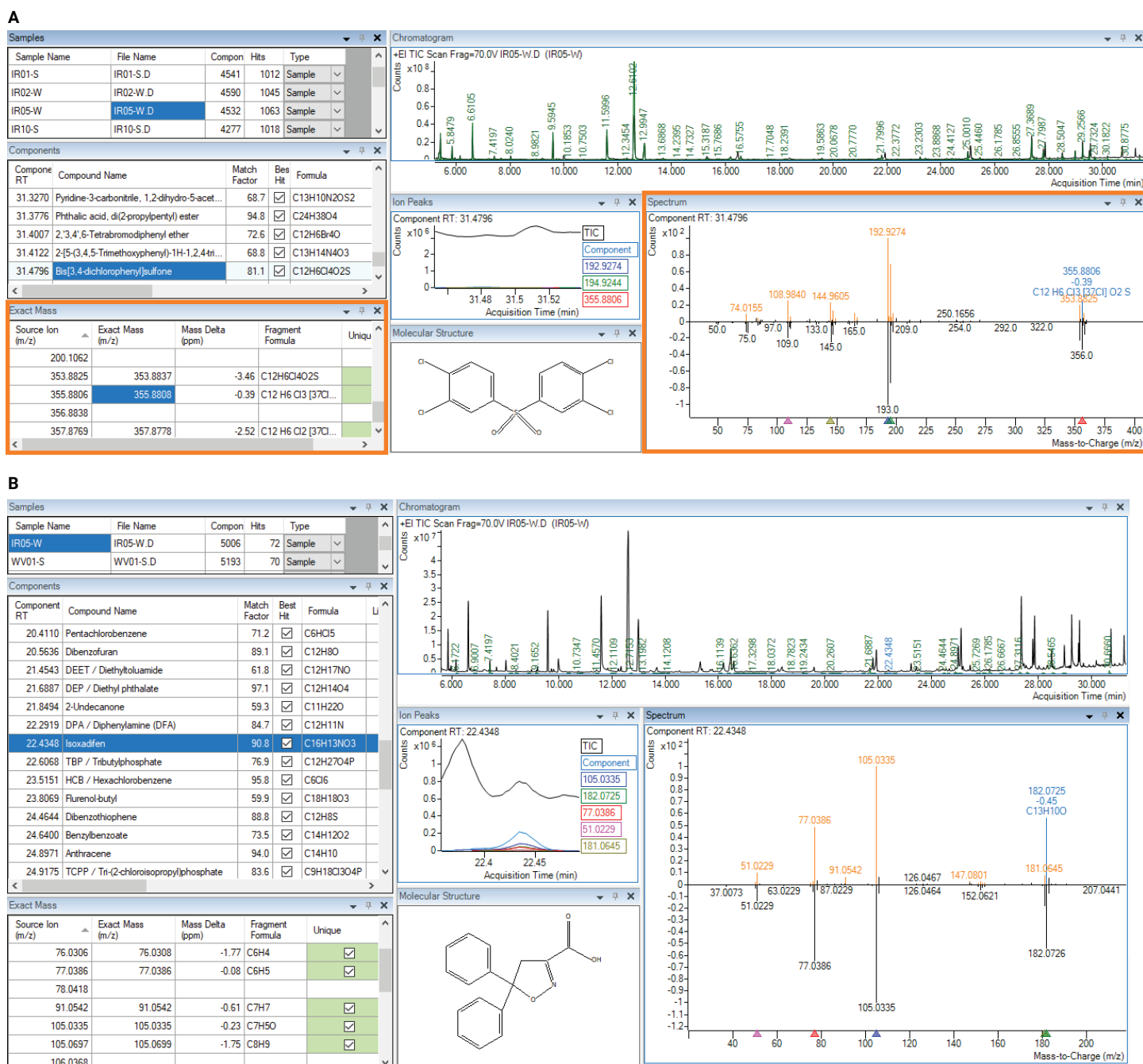
Figure 4. Examples of the contaminants identified in drinking water extracts using (A) NIST23 and (B) Agilent GC/Q-TOF Pesticide PCDL. The ExactMass tool (outlined in orange) helped to provide additional confirmation of unit mass library hits based on accurate mass. Compound ions are highlighted in the mirror plot when m/z corresponds to the library hit formula.
