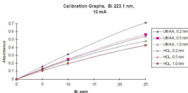
Figure 2. Comparison of Bi 223.1 nm calibration graphs using different design lamps and conditions.
