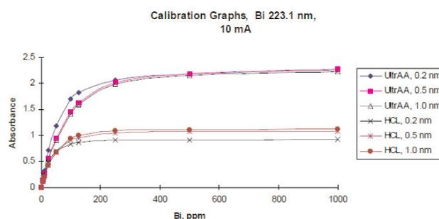
Figure 3. Comparison of Bi 223.1 nm calibration graphs using different design lamps and conditions.
