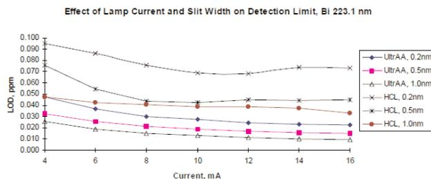
Figure 1. Effect of lamp current and slit width on detection limit, Bi 223.1 nm line.
