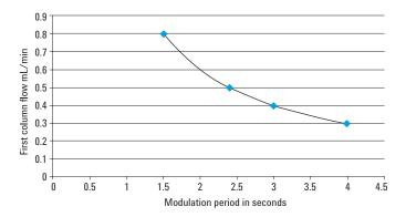
Figure 3. Relationship between modulation period and first dimension column flow rate.
