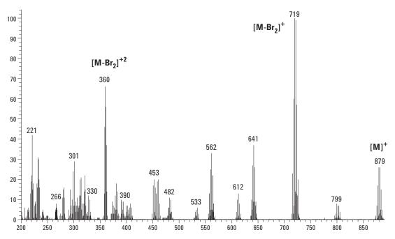
Figure 2. Electron impact ionization spectrum of a nonabromodiphenyl ether (PBDE-208) from 200 to 890 m/z.
