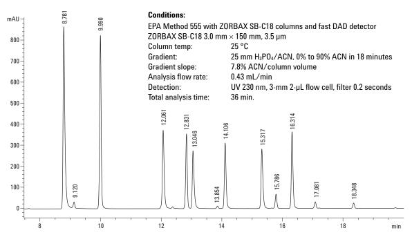
Figure 3. Gradient separation of herbicides on 3.0 × 150 mm, 3.5-μm ZORBAX SB-C18.
