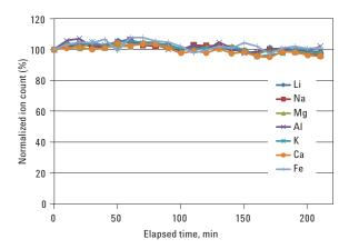
Figure 9. Four hours stability of cool plasma mode (100 ppt spiked into IPA).
