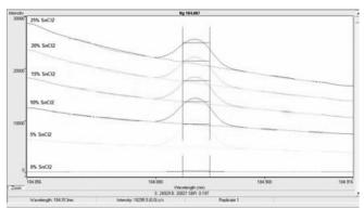
Figure 2. Signal traces of 50 μg/L Hg 184 nm at various SnCl<sub>2</sub> concentrations.
