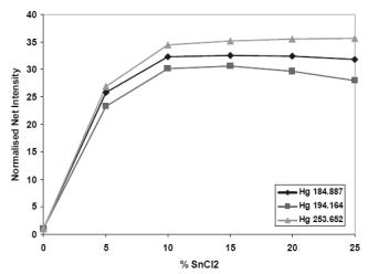
Figure 1. Effect of different  $SnCl_2$  concentrations on the signal intensity of 50  $\mu$ g/L Hg.
