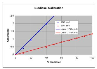
Figure 9. Quantitative measurement of biodiesel blends, B0, B10 to B90 and B10
