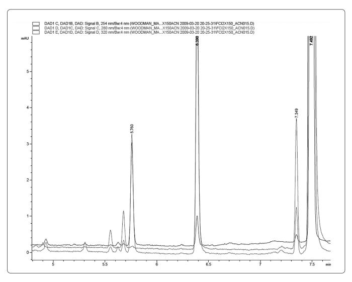
Figure 5. An expanded view of the acetonitrile separation using the same gradient slope on a 2.1 mm × 150 mm column rated for 1200 bar operating pressure. Agilent ZORBAX StableBond C18, 1.8 μm.
