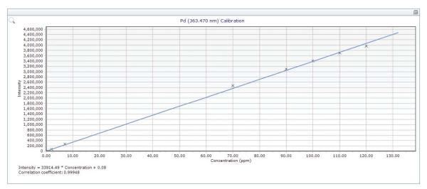
Figure 4. Calibration graph for Pd at the 363.469 nm wavelength
