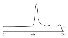
Figure 2. Chromatogram of a non-ionic surfactant
