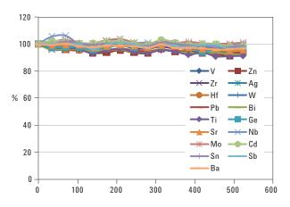
Figure 4. Nine hours stability of 7700s ICP-MS operating in He mode (100 ppt spike in 1% HNO $_3$ ).
