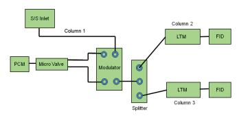
Figure 1. Diagram of the dual LTM GCxGC system.
