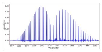
Figure 1. Sample spectrum displayed between 2250–2000 cm<sup>-1</sup> revealing the P (right) and R (left) branching of the C≡O stretching band centered at 2143.3 cm<sup>-1</sup>
