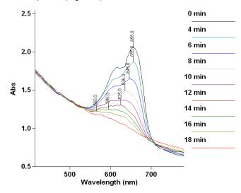
**Figure 2.** Scanning kinetics using fiber optics *in situ* of methylene blue under the exposure of a high-intensity UV lamp (Oriell 500 W Hg(Xe) lamp) over a period of 20 minutes within the range 400 to 800 nm. Labels refect maximum absorbance wavelengths
