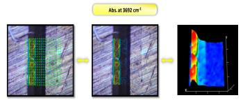
**Figure 3.** A feature image generated from a spectral peak that is unique to one layer of the paint chip (left), the same feature image shown without the spectral acquisition grid for clarity (center), and the 3-dimensional view of the feature image (right). These images were generated by plotting the intensity of the peak at 3692 cm<sup>-1</sup> in the spectrum from each pixel across the entire infrared map.
