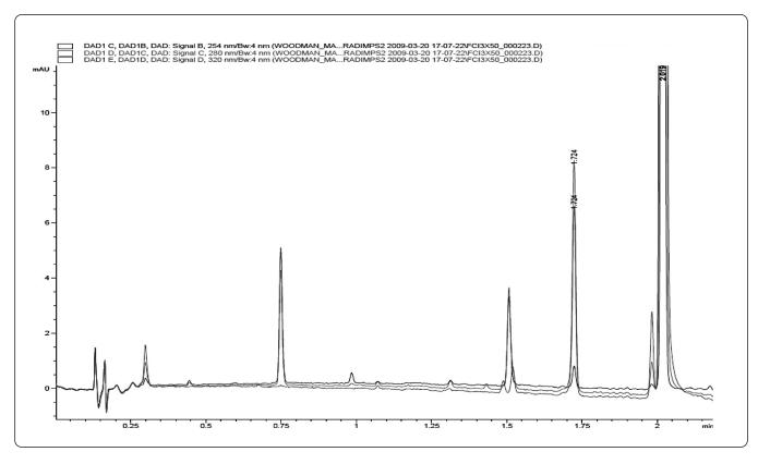
Figure 3. An expanded presentation of the chromatogram shown in Figure 2 based on the 3 mm  $\times$  50 mm gradient separation.
