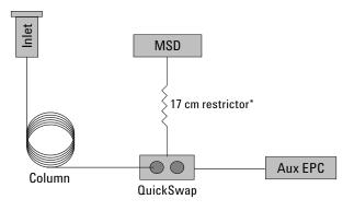
\*QuickSwap restrictor, P, and T are selected for desired flow to MSD, usually the maximum flow that the current application requires.
