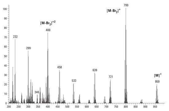
Figure 3. Electron impact ionization spectrum of the decabromodiphenyl ether (PBDE-209) from 200 to 1000 m/z.
