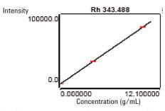
Figure 2. Calibration graph used for determination of the digested oil catalyst samples at the Rh 343.488 nm emission line.
