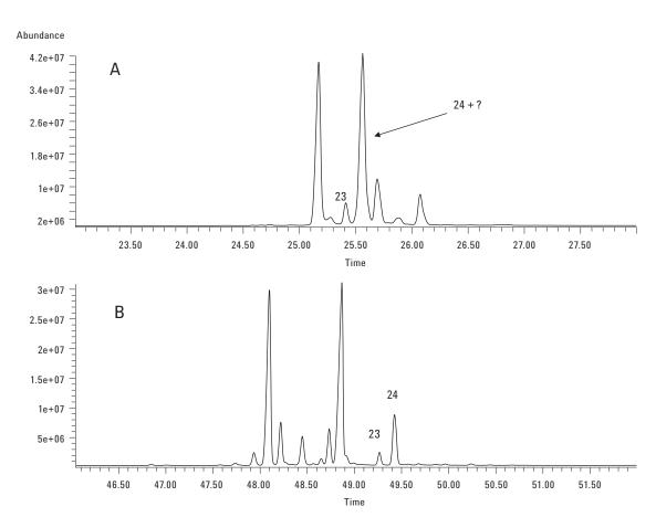
Figure 4. A) Separation of fraction 3 on the second-dimension column (Agilent J&W DB-17ms) using MS detection. Column 1 temperature = column 2 temperature: 50 °C (1 min) → 270 °C at 8 °C/min. Peaks: 23. Lyral 1; 24. Lyral 2. B) Separation of fraction 3 on the second-dimension column (Agilent J&W DB-17ms) using MS detection. Column 2 temperature: 50 °C (25 min) → 250 °C at 6 °C/min. Peaks: 23. Lyral 1; 24. Lyral 2.
