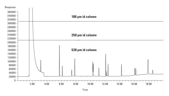
Figure 8. FID vent signal for three columns under optimal flow conditions. Only the 530-μm id column has a flow that exceeds the 1 mL/min flow to the MSD.
