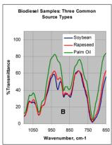
Figure 7. Detailed information from the base ester components used in the production of biodiesel methyl esters; hydroxyl (A) and unsaturation (B) functionalities
