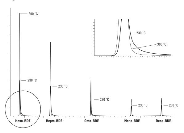
Figure 5. Overlaid RIC SIM acquisitions of five PBDEs at ion source temperatures of 230 °C and 300 °C. Insert is expanded view of hexa-BDE overlays near baseline.
