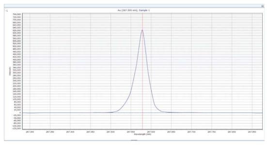
Figure 5. A typical PM sample spectrum for Au at the 267.595 nm wavelength
