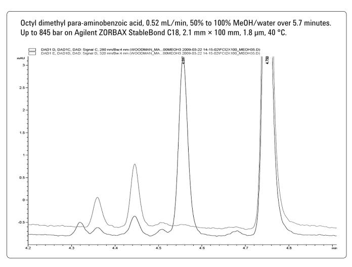
Figure 7. An expanded view of the small region of the chromatogram in Figure 6 showing a significant number of low concentration impurities. Conditions as in Figure 6. Estimated impurity concentrations for the smallest peaks in this figure are less than 0.02%.
