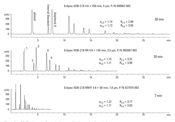
Figure 2. RRHT column configuration increased both speed and resolution.
