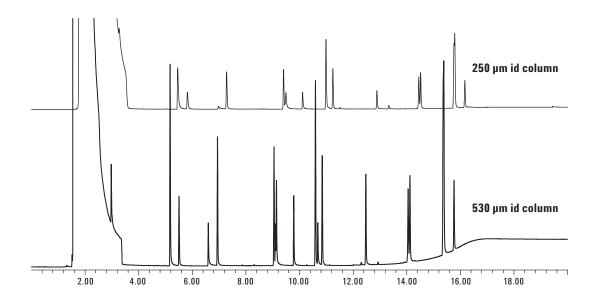
Figure 10. FID vent signals for the two largest columns operated at 2X optimal constant flow rate conditions.
