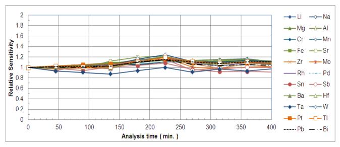
Figure 2: Signal stability of a representative selection of 22 elements spiked at 100 ppt in 20%  $NH_4OH$
