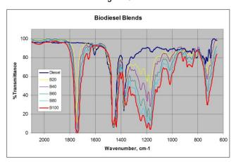
Figure 8. Measurement of biodiesel blends, experimental data from B0 (diesel fuel) to B100 (biodiesel) and intermediate biodiesel/diesel blends
