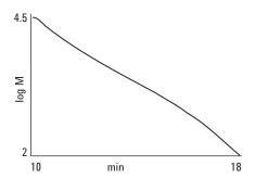
Figure 1. EasiVial calibration of PL aquagel-OH columns
