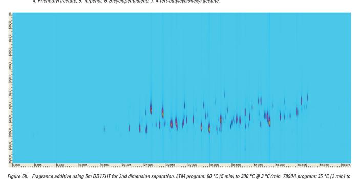
Figure 6b. Fragrance additive using 5m DB17HT for 2nd dimension separation. LTM program: 60 °C (5 min) to 300 °C @ 3 °C/min. 7890A program: 35 °C (2 min) to 280 °C @ 3 °C/min.
