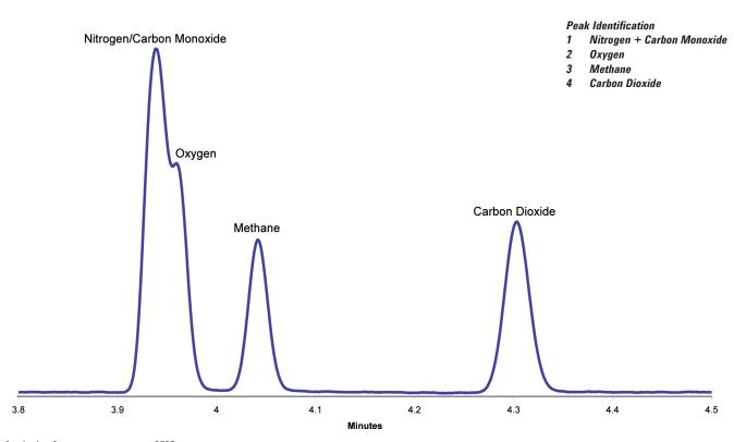
Analysis of permanent gases at 35°C
