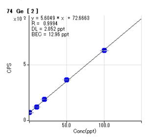
Figure 3. 74Ge calibration curve obtained using high energy He mode
