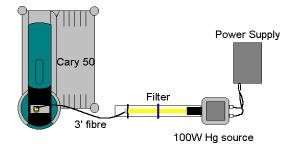
Figure 4. Setup of apparatus used for irradiating sample
