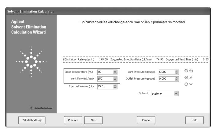
Figure 3. The calculator calculates the injection rate and vent time according to the selected inlet temperature and vent flow.
