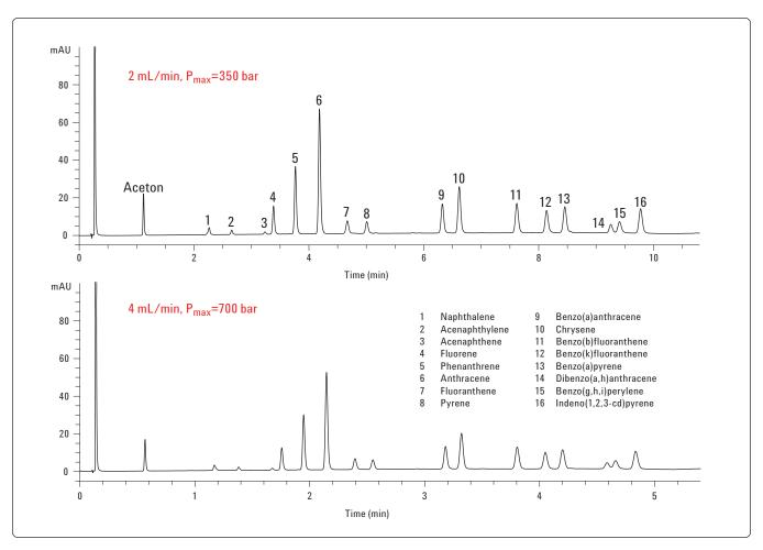
Figure 1 Analysis of 16 PAHs on the 1290 Infinity LC. Sample: standard solution of 16 PAHs, 50  $\mu$ g/mL each.
