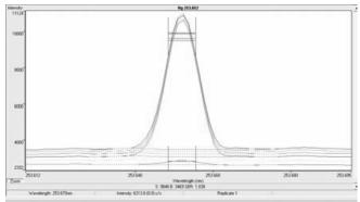
Figure 4. Signal traces of 50 μg/L Hg 253 nm at various SnCl<sub>2</sub> concentrations.
