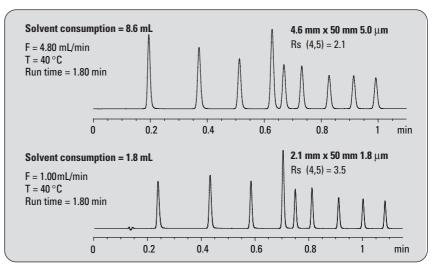
Figure 3 Analysis with 1.8-μm particle column vs. 5.0 μm particle column.
