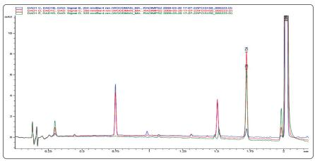
Figure 2 Initial separation conditions showing a need for greater resolution and selectivity. Sample: Octyl dimethyl para-aminobenzoate, 1 mg/mL. Gradient: 1.5 mL/min, 40% to 90% ACN/water over 2 minutes. Up to 460 bar on ZORBAX StableBond RRHT C18, 3 mm  $\times$  50 mm, 1.8  $\mu$ m, 40 °C. 0.75 minute retention: 4-amino-benzoic acid; 2.1 minute retention: Octyl dimethyl para-aminobenzoate.
