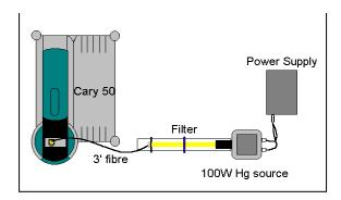
Figure 2. Setup of apparatus used for irradiating sample
