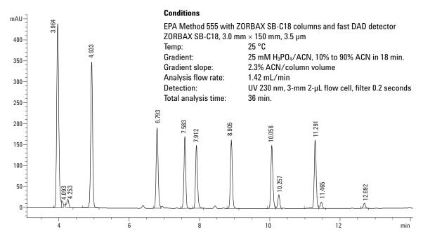
Figure 5. Reduced slope gradient separation of herbicides on 3.0 × 150 mm, 3.5-μm ZORBAX SB-C18.
