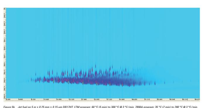
Figure 5b. Jet fuel on 5 m × 0.25 mm × 0.15 µm DB17HT, LTM program: 60 °C (5 min) to 300 °C @ 3 °C/min. 7890A program: 35 °C (2 min) to 280 °C @ 3 °C/min.
