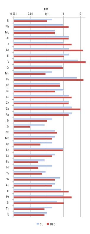
Figure 6. 7700s ICP-MS DLs and BECs in undiluted IPA.
