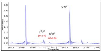
**Figure 3.** Expanded view of the same spectrum of carbon monoxide between 2117 and 2109 cm $^{-1}$ , illustrating transitions of the  $C^{12}O^{16}$ ,  $C^{13}O^{16}$  and  $C^{12}O^{18}$  isotopomers
