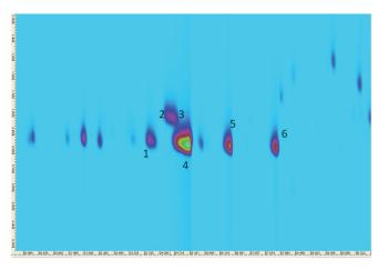
Figure 7a. Lime oil on the 7 m INNOWax. LTM program: 55 °C (3 min) to 270 °C @ 5 °C/min. 7890A program: 35 °C (2 min) to 280 °C @ 3 °C/min. 1. Alpha Pinene, 2. Limonene, 3. 2,6 dimethyl 7-octen-2-ol, 4. Phenethyl acetate, 5. Terpenol, 6. Bicyclopentadiene, 7. 4-tert-butylcyclohexyl acetate 1.beta pinene, 2. 1,4 Cineol, 3. m-cymene, 4. Limonene, 5. Terpinen, 6. Terpinolen
