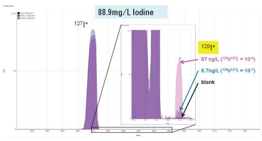
Figure 4. Overlaid spectra of 88.9 mg/L <sup>127</sup>| blank, NIST 3231 Level I (87 ng/L <sup>129</sup>I), and the intermediate standard (8.7 ng/L <sup>129</sup>I)
