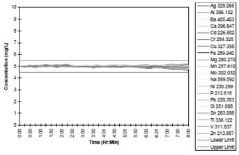
Figure 1. Stability of the Vista-PRO radial instrument over 8 hours. Results remained within ±10% for all elements in the 5 mg/L S21 kerosene solution without internal standardization or recalibration.
