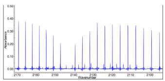
Figure 2. Spectrum of C≡0 between 2170–2095 cm<sup>-1</sup> highlighting the fine detail of the R branches of C¹³O¹6
