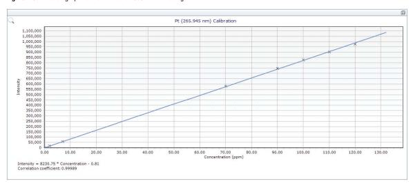
Figure 3. Calibration graph for Pt at the 265.945 nm wavelength
