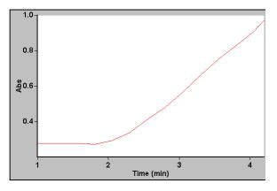
Figure 3. Absorbance(510 nm) vs time during irradiation with 366 nm Hg light
