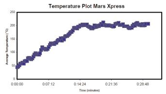
Figure 1. MarsXpress digestion temperature profile.
