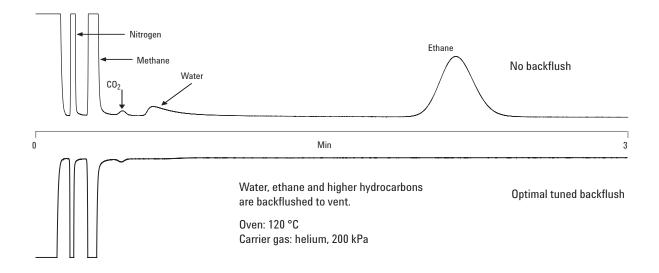
Figure 2. Backflush of water and ethane.
