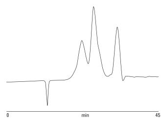
Figure 3. Separation of fullerene using an Agilent PLgel 10 µm analytical packing to predict a preparative scale separation using the same packing.
