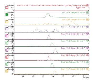
Figure 2. Chromatogram of a blank injection (top) followed by the same blank spiked with Tergitol NP-10, Tergitol 15-S-7, and Tergitol 15-S-9.
