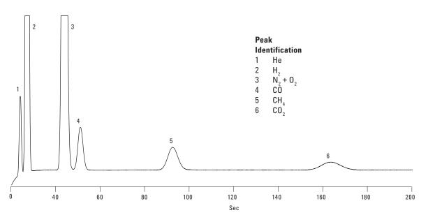
Figure 1. Excellent baseline separation of a gas sample on a COX column.
