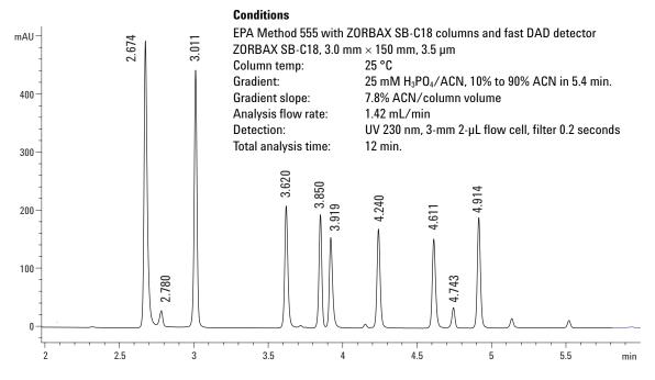
Figure 4. High speed gradient separation of herbicides on 3.0  $\times$  150 mm, 3.5- $\mu$ m ZORBAX SB-C18.
