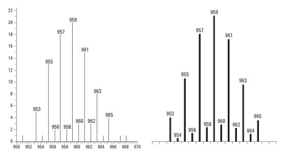
Figure 4. Experimental spectrum of the decabromodiphenyl ether (PBDE-209) molecular ion cluster [M]<sup>+</sup> versus theory.
