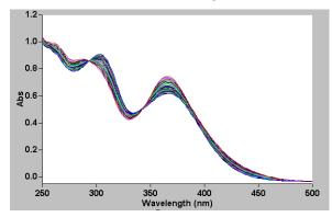
Figure 6. Change in absorption spectra of 1a in CH3CN during irradiation with Hg light
