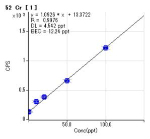
Figure 1. 52Cr calibration curve obtained using He mode and cool plasma
