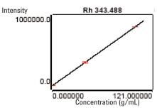
Figure 1. Calibration graph used for the determination of the aqueous sample at the Rh 343.488 nm emission line.
