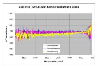
**Figure 2.** 100% Baseline performance; spectra from long, medium and short pathlengths presented with an average SNR of 8000:1 (2100 cm $^{-1}$  to 1100 cm $^{-1}$ )
