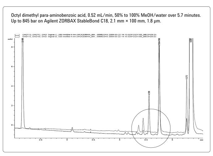
Figure 6. Separation of the sample mixture on a 2.1 mm × 100 mm Agilent ZORBAX StableBond C18, using methanol as the organic phase. Flow rate 0.52 mL/min gradient time 5.7 min, for a gradient of 5% to 100% methanol
