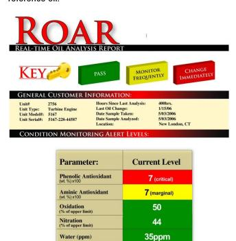
Figure 3. Agilent 5500t FTIR software presents the user with the specific concentration of phenolic and aminic antioxidants as well as crucial information about oxidation by-products and level of water contamination
