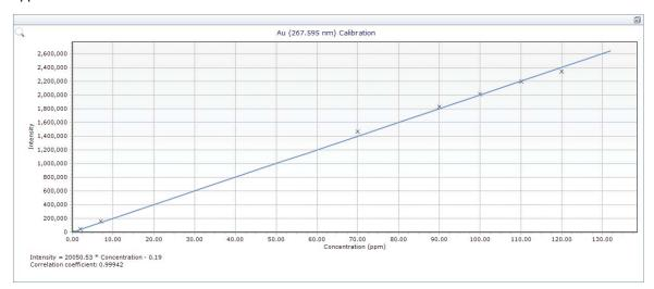
Figure 2 Calibration graph for Au at the 267.595 nm wavelength
