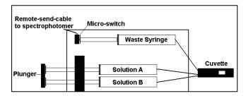
Figure 2. Schematic of Rapid Mix Accessory
