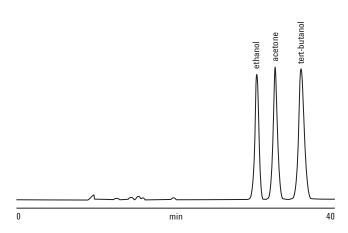
Figure 1. Separation of different aliphatic compounds on an Agilent Hi-Plex H column.
