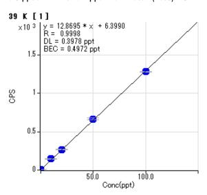
Figure 2. 39K calibration curve obtained using NH<sub>3</sub> mode and cool plasma
