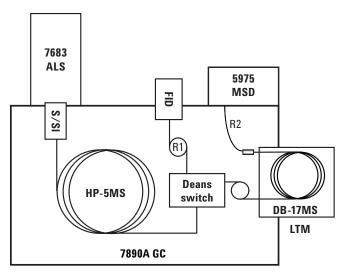
Figure 2. System configuration.
