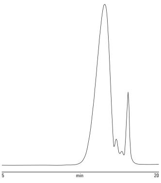
Figure 1. Raw data chromatogram of sodium polyacrylate
