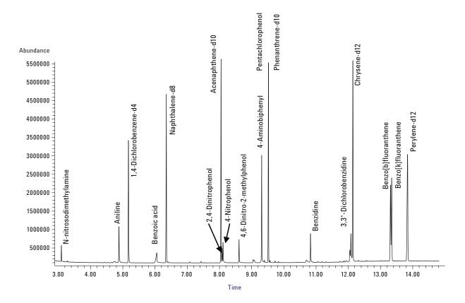
Figure 4. Reference chromatogram for Fast 8270 method.
