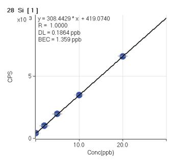
Figure 3. 7700s ICP-MS H<sub>2</sub> mode calibration for <sup>28</sup>Si in 1% HNO<sub>2</sub>.
