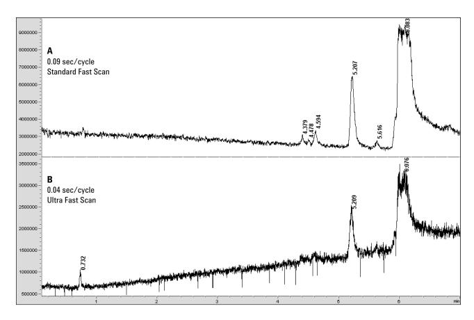
Figure 3. The total ion chromatograms (TICs) corresponding to the highest acquisition speed of the Standard Fast Scan mode (A) and the Ultra Fast Scan mode (B).
