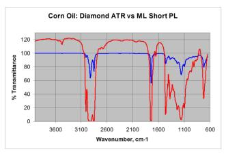
Figure 4. Comparison of the effective pathlength of a diamond ATR integrated system with the short fixed pathlength (~30  $\mu$ m) transmission spectrum for corn oil
