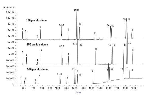
Figure 5. Constant pressure mode analysis with three different column dimensions; 0.5-µL splitless injections of 80-ppm semi-volatiles test sample, with flow conditions from Table 2.
