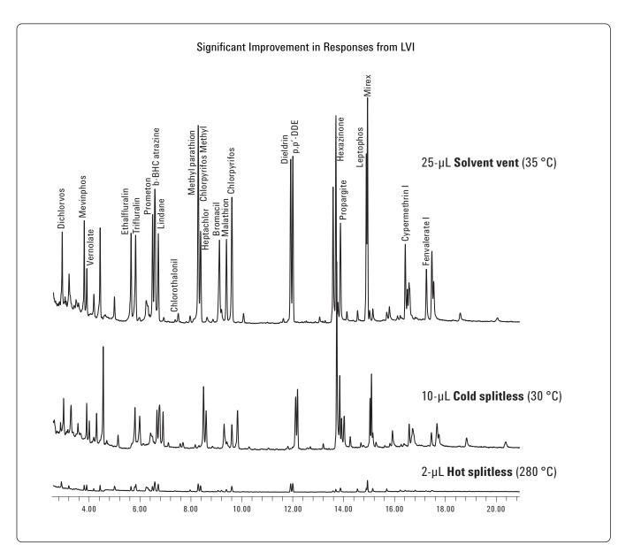
Figure 5. Overlay of total ion chromatograms (TICs) from three injection modes, plotted on the same scale.
