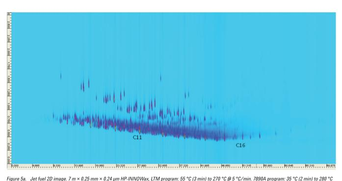
Figure 5a. Jet fuel 2D image. 7 m × 0.25 mm × 0.24 µm HP-INNOWax, LTM program: 55 °C (3 min) to 270 °C @ 5 °C/min. 7890A program: 35 °C (2 min) to 280 °C @ 3 °C/min.
