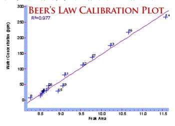
**Figure 2.** The calibration plot of KF water values ( ppm) versus peak absorbance area for water in turbine oil using a Beer's Law peak area method
