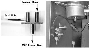
Figure 2. QuickSwap is pictured on the left showing permanent (Aux EPC In) and temporary connections. A picture of a normal QuickSwap installation is shown on the right.
