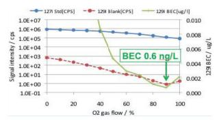
Figure 1. Profile of <sup>127</sup>I sensitivity, m/z 129 background and <sup>129</sup>I BEC versus oxygen flow rate
