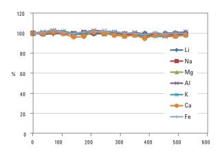
Figure 8. Nine hours stability of cool plasma mode (100 ppt spike in 1% HNO $_3$ ).
