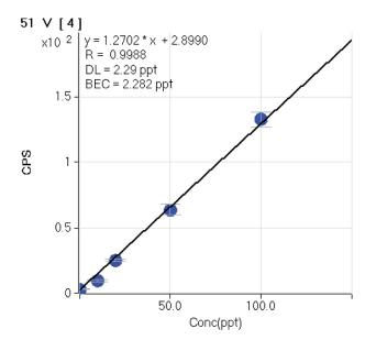
Figure 5. Vanadium calibration in undiluted HCl, using NH<sub>3</sub> mode.
