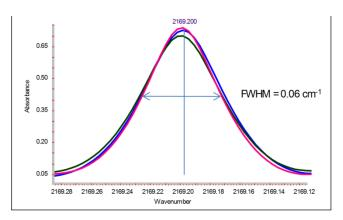
**Figure 4.** Spectra of three replicates of the R-6 transition of  $C^{12}O^{16}$ . Such spectra were used to calculate the wavelength precision, accuracy and resolution of the Agilent Cary 670 FTIR spectrometer
