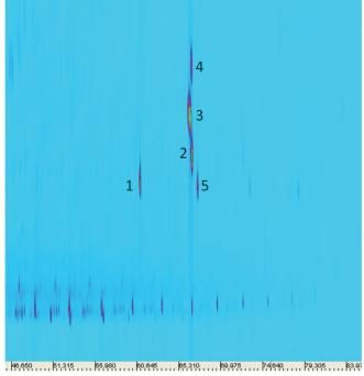
Figure 8. Separation of C16 and C18 fatty acid methyl esters in B20 biodiesel on a 5 m × 0.25 mm × 0.15 µm LTM INNOWax column in the 2nd dimension. LTM program: 30 °C (0 min) to 270 °C (5 min) @ 3 °C/min. 1. C16:0, 2. C18:1, 3. C18:3, 4. C18:3, 5. C18:0.
