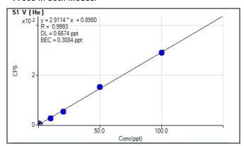
Figure 1a: Calibration plot showing spikes at 0, 10, 20, 50 and 100 ppt for V in 20%  $\,NH_4OH\,$
