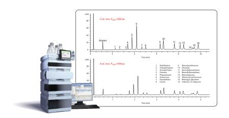
The Agilent 1290 Infinity LC has a broader power range (the combination of pressure and flow capabilities) than any other commercially available system. This is extremely useful for method transfer from one (U)HPLC to the Agilent 1290 Infinity LC system and allows the analyst to develop methods that are impossible to run on these other systems.
