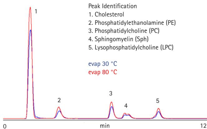
**Figure 2.** Separation of a 100 µg/mL polar lipid mixture at ambient temperature with the Varian ELSD.
