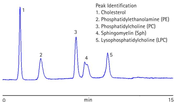
**Figure 3.** Excellent sensitivity of the Varian ELSD to polar lipids resulting from very low signal to noise ratios.
