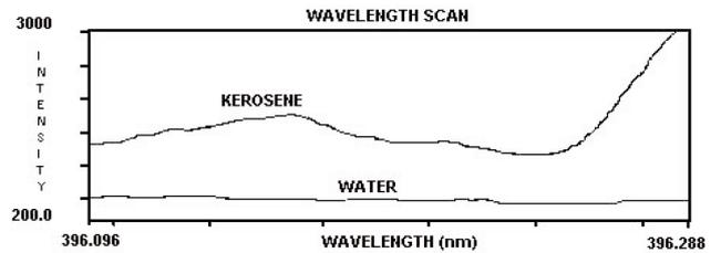
Figure 4. Background emission of kerosene blank and water blank at Al 396.152 nm.
