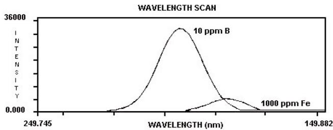
Figure 1. The effect of 1000 ppm Fe on 10 ppm B at the B 249.773 nm line.
