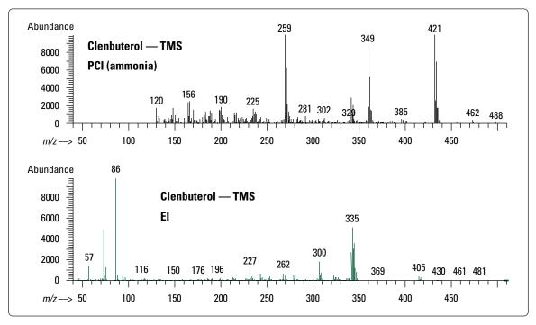
Figure 2. El and PCI (ammonia) spectra for clenbuterol — TMS.
