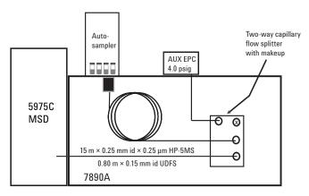
Figure 1. Schematic diagram of GC-MS system.
