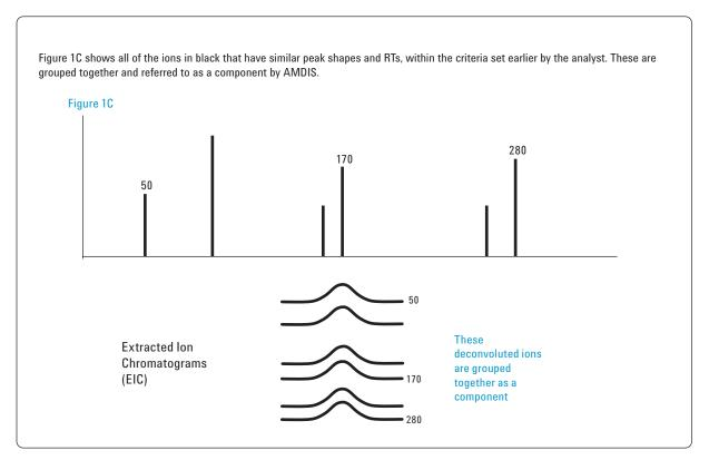
Figure 1A-1C. Simplified deconvolution process (continued).
