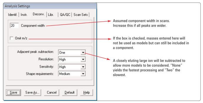
Figure 4. AMDIS deconvolution settings.
