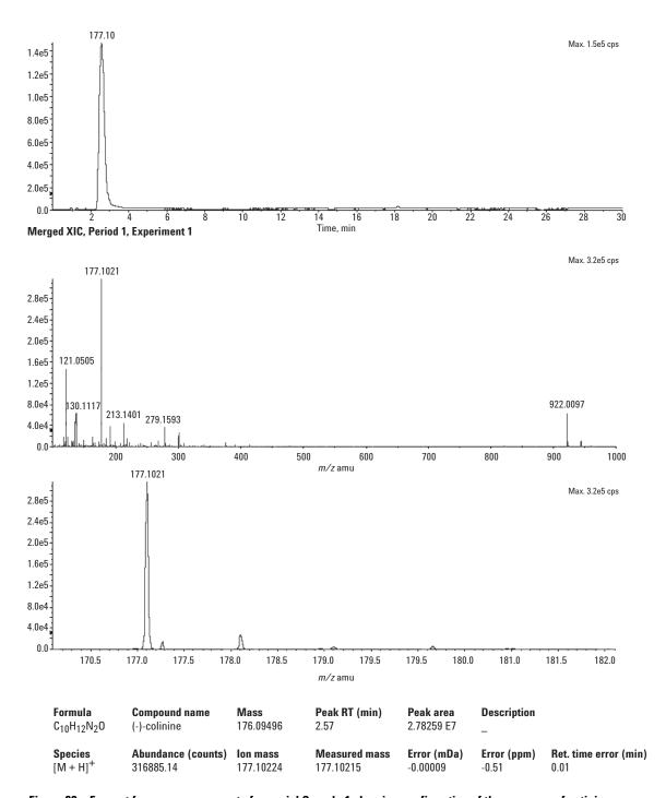
Figure 22. Excerpt from screener report of coronial Sample 1 showing confirmation of the presence of cotinine.
