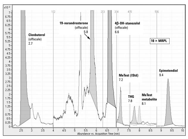
Figure 2. Chromatographic profile of 10 × MRPL extract in urine.
