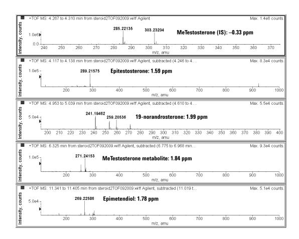
Figure 7. Spectra from 2 ng/mL urine extract (1 ng/mL 19-norandrosterone) (240/120 pg on-column) [see Figure 6].
