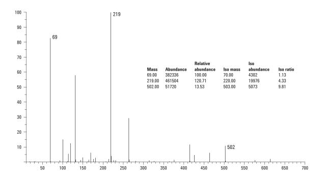
Figure 1. Autotune results for an ion source temperature of 230  $^{\circ}\text{C}.$
