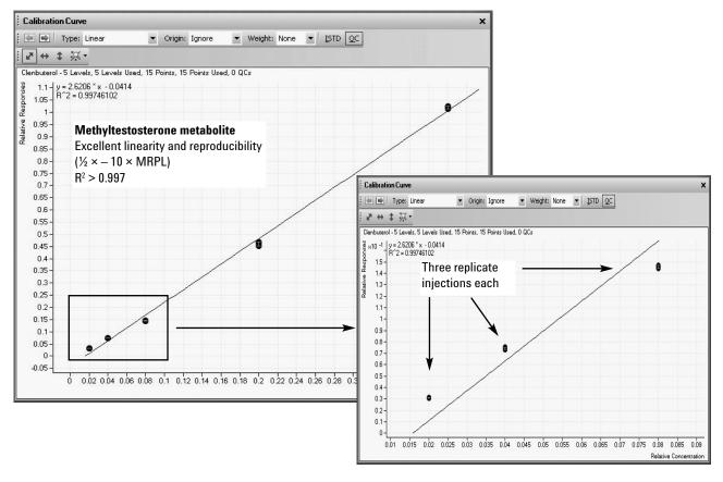
Figure 5a. Linearity of methyltestosterone metabolite.
