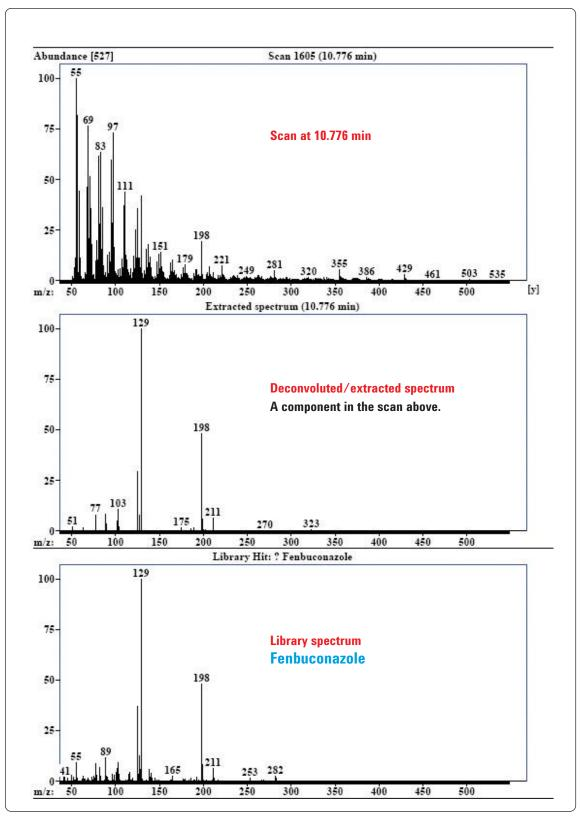
Figure 2. Comparison of raw, deconvoluted, and library spectra.
