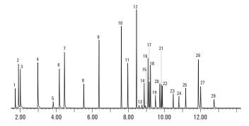
Figure 3. Chromatogram of forensic/toxicology analyzer checkout standard (5 ng checkout standards on column) using Agilent Ultra Inert single taper splitless liner with wool (p/n 5190-2293) by GC/MS. See Table 1 for instrument condition. Satisfactory peaks shape achieved for all of analytes
