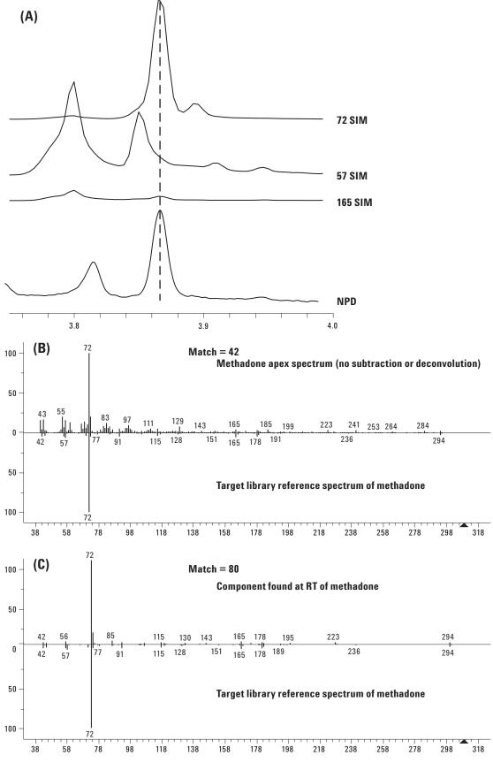
Figure 5. (A) Methadone SIM and NPD chromatograms.
