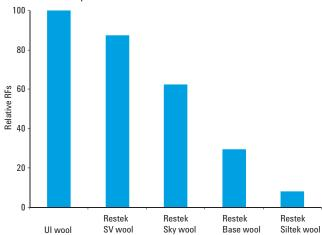
Figure 4. Sensitive compound response (Temazepam) comparison for Ultra Inert liner with wool (p/n 5190-2293) and other equivalent liners. RF calculation was based on the average RF of 0.5 ng and 5 ng standard on column. Ultra Inert liner average RF value was set to 100% and other liners average RF values were scaled.
