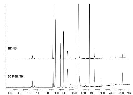
Figure 8. Comparison of chromatogram on GC system 1 with GC-MSD system after retention time locking, Constant Pressure Mode
