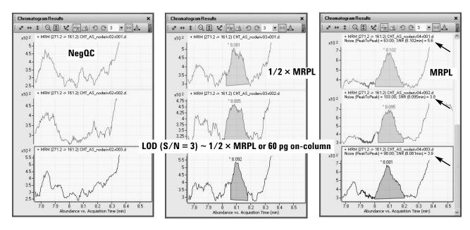
Figure 5b. Estimate of LOD for methyltestosterone metabolite.
