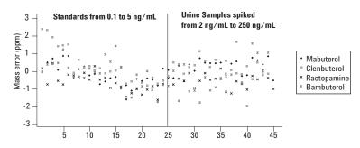
Figure 4. Mass Accuracy on an 18-hour sequence for the investigated  $\Omega_2$ -agonists.
