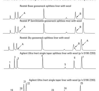
Figure 2. Chromatographic problems for drug of abuse compounds shown on GC/MS SIM chromatograms when using other equivalent liners and their comparison with chromatograms obtained by Ultra Inert liners with wool. See Table 3 for peaks identification and Table 1 for instrument conditions. 5 ng checkout standards on column. A) Broad or distorted peak, B) ghosting shoulder, C) poor sensitivity
