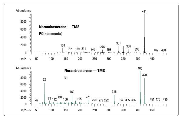
Figure 3. El and PCI (ammonia) spectra for norandrosterone — TMS.
