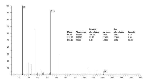
Figure 2. Autotune results for an ion source temperature of 300  $^{\circ}$ C.
