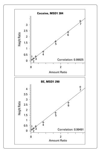
Figure 4. Calibration curves for cocaine and BE.
