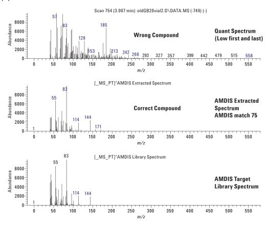
Figure 8C. Three meprobamate spectra presented in QEdit for comparison during data review using DRS A.04. (continued)
