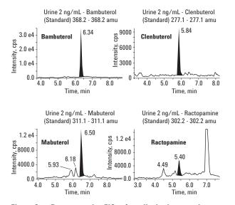
Figure 2. Representative EICs of a spiked urine sample at the 2 ng/mL level.
