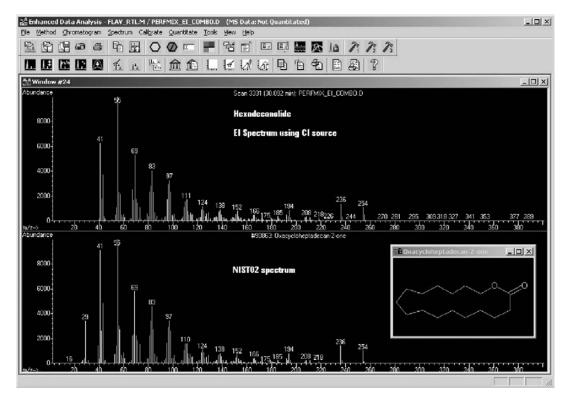
Figure 3. Acquired El spectrum compared to the NISTO2 library reference spectrum.
