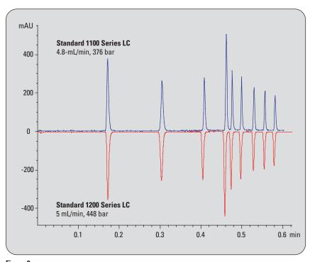
Standard Agilent 1200 Series RRLC system vs. Agilent 1100 Series LC system: analysis of phenone mix on 4.6-mm ID column packed with 1.8-µm particles.
