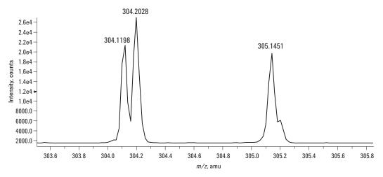
Figure 14. Mass spectrum 304 – 305 amu for peak at 11.9 minutes – no match of mass for cocaine.
