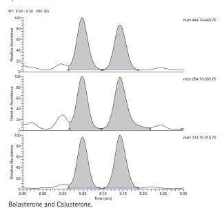
Figure 1. Mass spectral information of the anabolic steroids.
