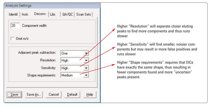
Figure 5. AMDIS deconvolution settings.
