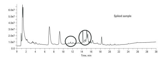
Figure 10. TIC of Neat Urine with 100 ng/mL spike of cocaine, benzoylecognine, flunitrazepam, and 7-aminoflunitrazepam.
