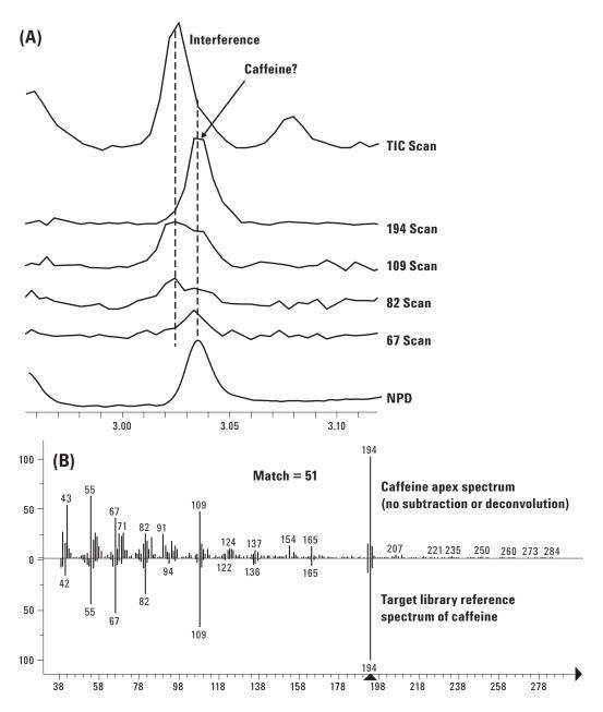
Figure 6. (A) TIC, scan EICs, and NPD signals for caffeine.
