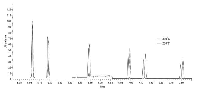
Figure 4. Overlaid RTICC of six PCBs acquired in SIM at source temperatures of 230 °C and 300 °C. From left to right, or earlier to later, in the chromatogram the PCBs consist of a Cl<sub>3</sub>-Biphenyl, Cl<sub>4</sub>-B, Cl<sub>5</sub>-B, Cl<sub>6</sub>-B, another Cl<sub>6</sub>-B and a Cl<sub>7</sub>-B.
