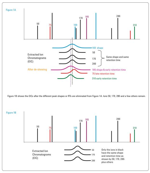
Figure 1A-1C. Simplified deconvolution process (continued).
