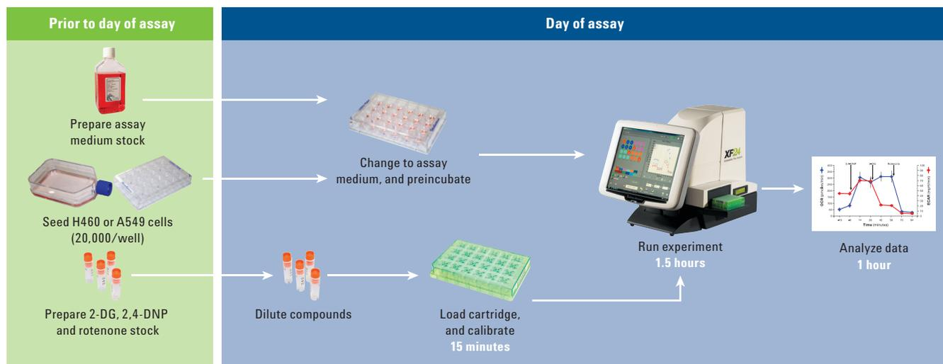
Figure 2. Flow chart of the XF assay.
