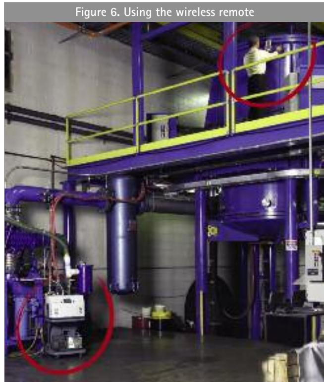
indicating the trend and relative size of the leak. Large systems, in which two technicians were previously required, can now be tested by one technician, thereby reducing labor costs.
