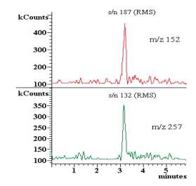
Figure 1. MRM Chromatograms of CAP (100 fg/JJL)
