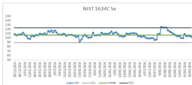
**Figure 2.** Quality control charts for As (top) and Se (bottom) based on a total of 147 separate measurements of NIST 1634c taken over 12 months
