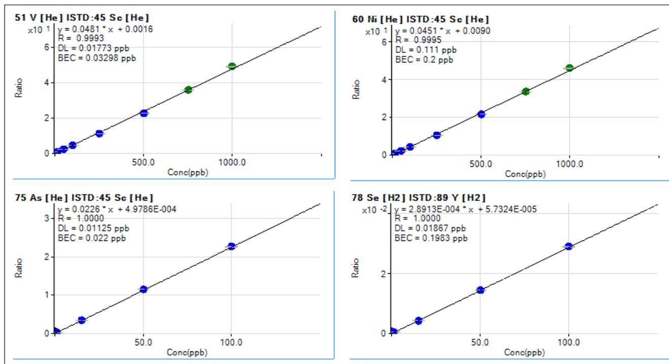
Figure 1. Calibration curves of V, Ni, As, and Se
