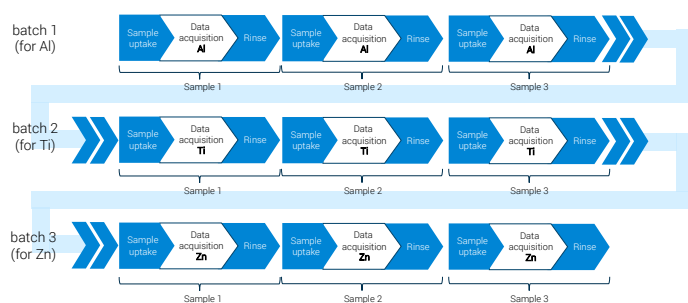
Figure 1A. Conventional spICP-MS method.
