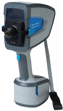
The Agilent 4300 Handheld FTIR fitted with the specular 45° external reflectance interface used in this study
