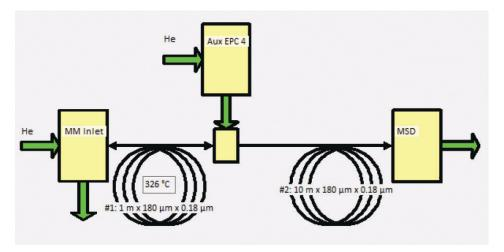
Figure 2. Backflush setup.
