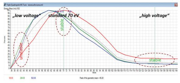
**Figure 3.** As the result of varying electron energy from 35 eV to 145 eV, signal intensity and stability changes. At 130 eV, the signal was stable, and produced approximately 10-20 % of the response obtained at the standard 70 eV operation, eliminating the saturation of the high-concentration species. Note that at 35 eV, the signal is significantly reduced, but the response is not stable. This is characteristic for most filaments.
