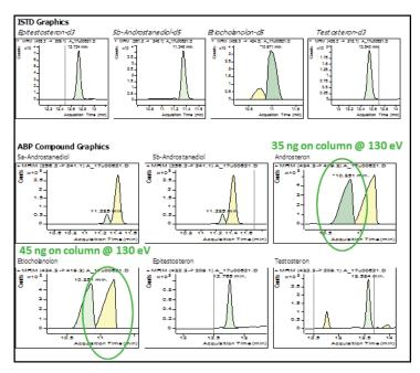
Figure5B. Suppressed response at 130 eV electron energy prevents saturation, and gives the expected look for chromatographically overloaded peaks.
