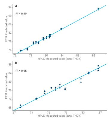
**Figure 3.** PLS-1 calibration model plot showing the correlation of potency value measured between the reference technique HPLC on the x-axis, and the FTIR-predicted value on the y-axis. A) Distillates sample calibration plot; B) concentrates sample calibration plot.
