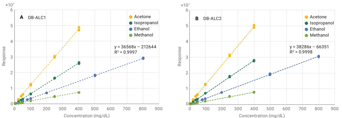
**Figure 2.** Calibration curves for ethanol, acetone, isopropanol, and methanol show excellent linearity on both column/detector pairs. The ethanol calibration shows good agreement between both channels.
