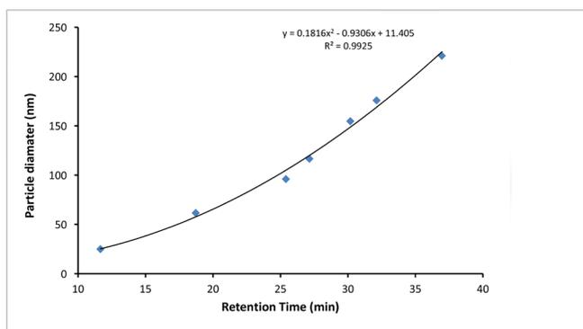
**Figure 1.** Calibration curve for silica nanoparticles
