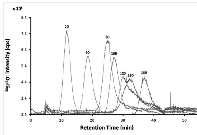
**Figure 3.** Overlaid FFF-ICP-QQQ fractograms of individual near-monodisperse NanoXact silica particle solutions. Numbers above the peaks represent the nominal size of each fraction in nm. Reproduced by permission of The Royal Society of Chemistry (RSC)
