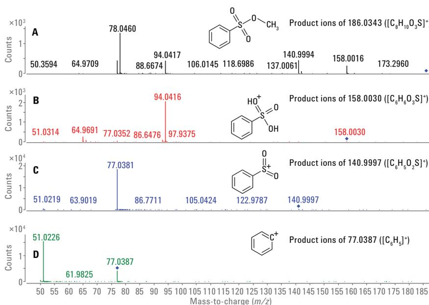
Figure 7. MS/MS data of EBS (dissociated ions of most abundant fragmented ions).
