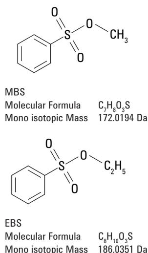
Figure 1. Molecular structure and formula for MBS and EBS.
