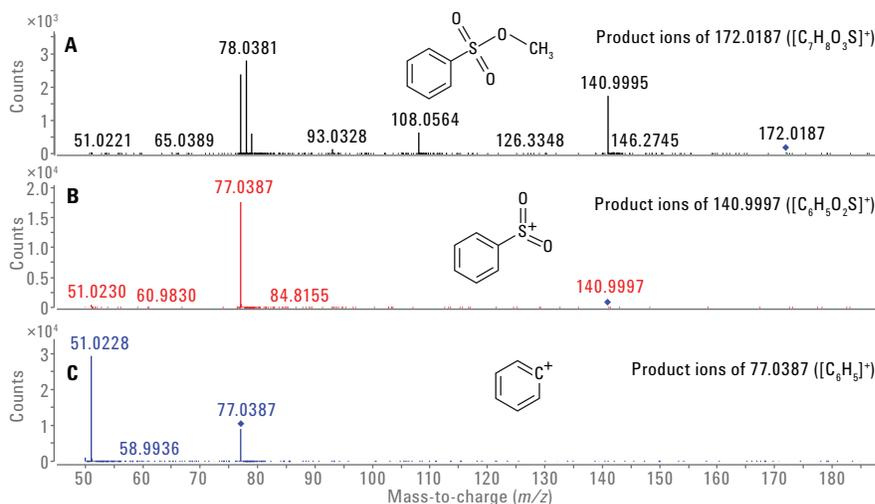
Figure 6. MS/MS data of MBS (dissociated ions of most abundant fragmented ions).
