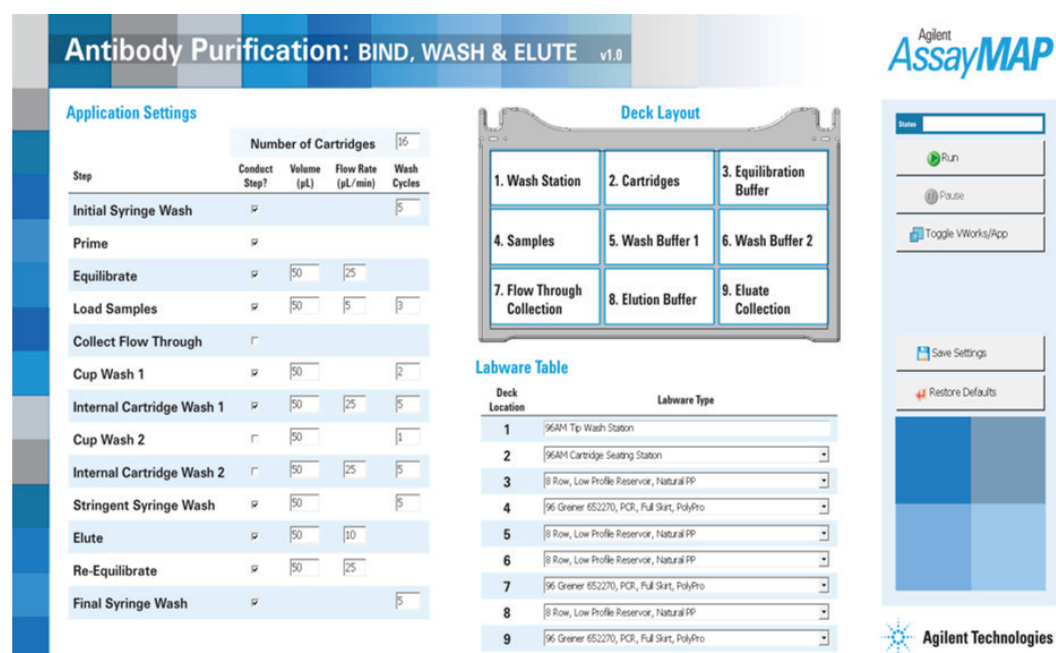
Figure 1. Agilent AssayMAP application interface showing the Antibody Purification protocol adapted for the cell surface protein isolation.
