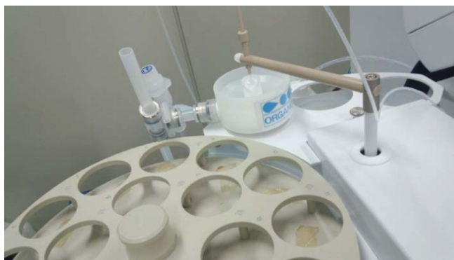
Figure 1. Photograph of the Organo flowing rinse port kit fitted to the Agilent I-AS autosampler
