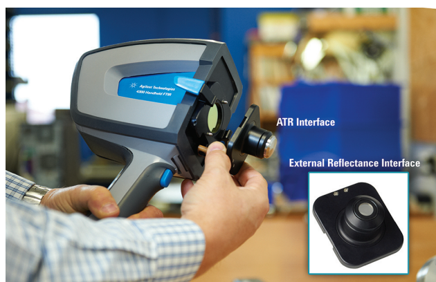
Figure 2. Agilent 4300 Handheld FTIR with diamond ATR and external reflectance sample interfaces used for measurement of PET. Sample interfaces are instantly interchangeable with no realignment necessary.
