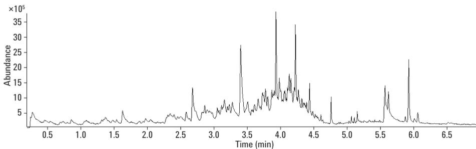
Figure 5. TIC of diesel by CTS sampling.
