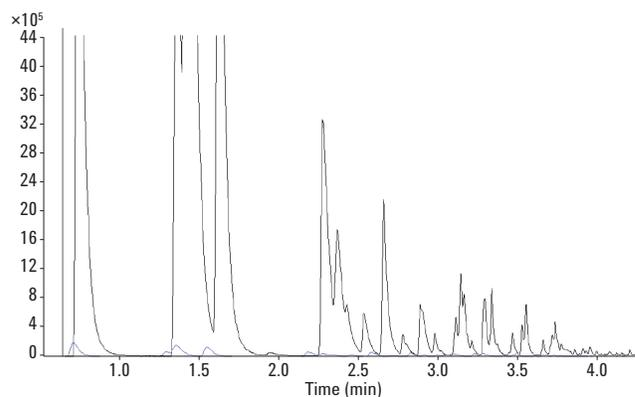
Figure 3. Mass chromatograms of fingerprints of gasoline ( $m/z$  91). Gasoline standards (black) and fire debris caused by gasoline (blue).
