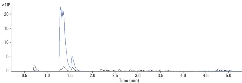
Figure 4. Mass chromatogram of banana oil and gasoline ( $m/z$  91), banana oil (blue), gasoline (black). Both are samples from the field.
