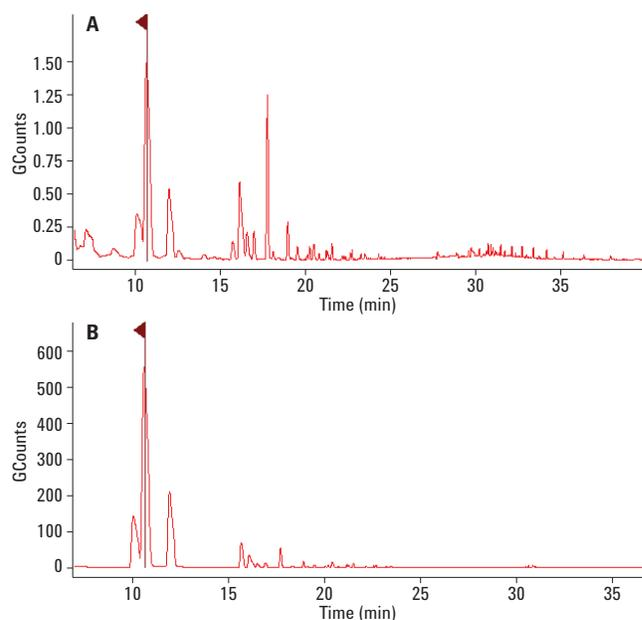
Figure 2. SPME results for 97# gasoline. A) TIC and B) EIC of  $m/z$  91.
