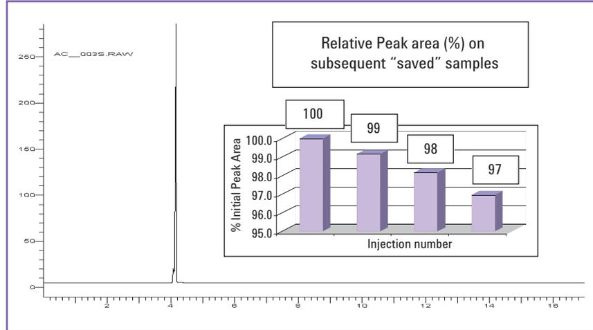
**Figure 4: Re-collection and repeat analysis of desorbed toluene**
