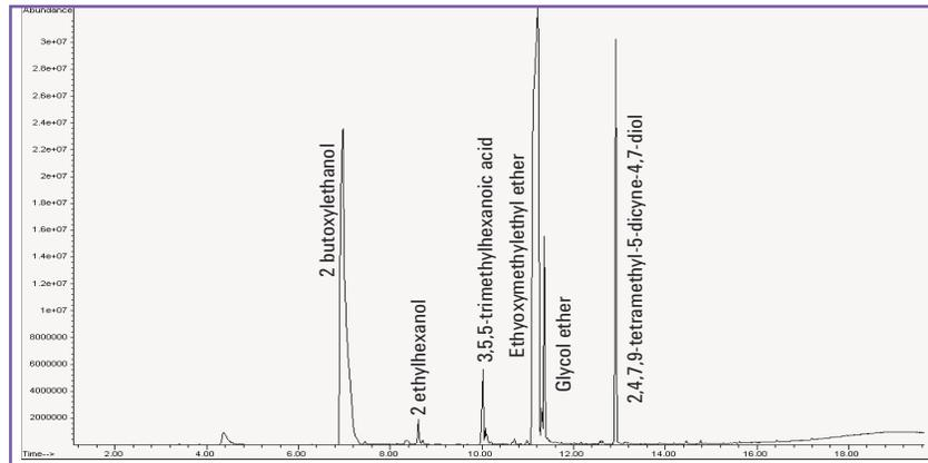
**Figure 7: Direct desorption of (semi) volatile organics from paint**
