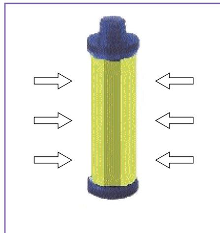
**Figure 3: Radial diffusive samplers**
