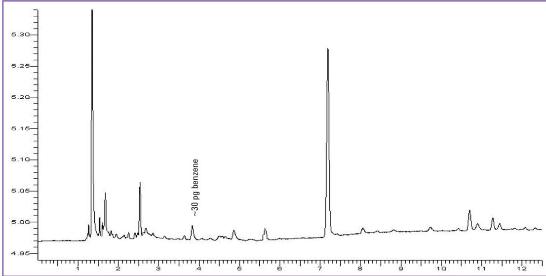
**Figure 1: 30 pg of benzene from a sorbent tube. Equivalent to 10 ppt in 1 L of air**
