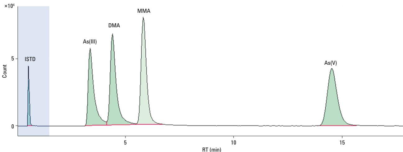
Figure 1. Chromatographic separation of arsenic standards at 5 ng/g.
