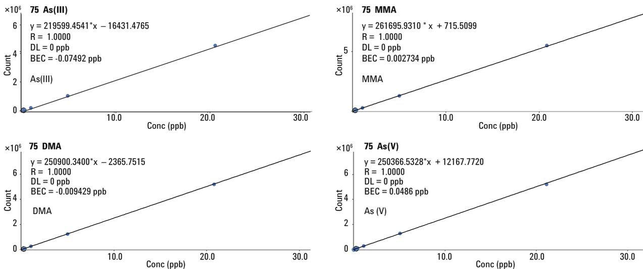
Figure 2. Calibration curves for the EAM 4:11 method.
