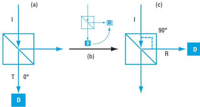
**Figure 3.** (a) CBS sample and detector (D) orientation for transmission measurement. (b) The detector is rotated around the sample in the plane of incidence so that for reflection measurements (c) the detector is at 90° to the incident beam and sample. NOTE: The sample does not move.
