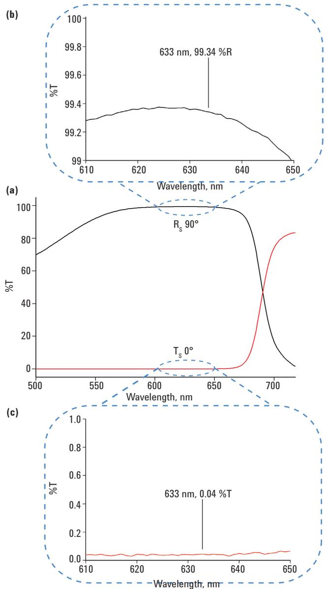
**Figure 4.** (a) Transmission and reflection spectra for s-polarized light measured on a CBS sample in the Cary 7000 UMS. (b) Reflection spectrum zoomed in around 633 nm. (c) Transmission spectrum zoomed in around 633 nm.
