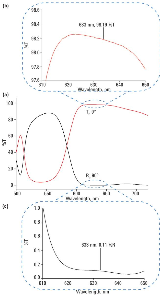
**Figure 5.** (a) Transmission and reflection spectra for p-polarized light measured on a CBS sample in the Cary 7000 UMS. (b) Transmission spectrum zoomed in around 633 nm. (c) Reflection spectrum zoomed in around 633 nm.
