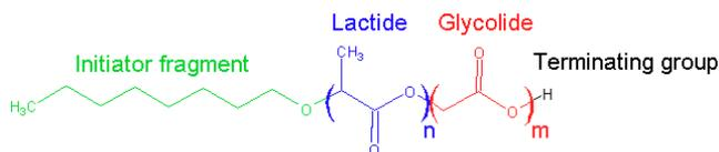
**Figure 18.** Structure of poly(lactide-co-glycolide) random copolymers
