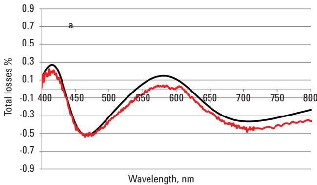
further confirmation that thickness non-uniformity does not affect total losses when T and R measurements are acquired at the same point of the sample.
