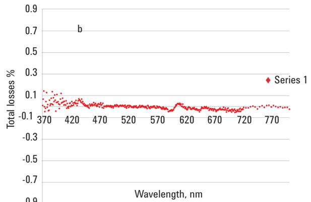
**Figure 2.** (a) Comparison of  $TL^{(s)}(\lambda) = 100\% - T^{(s)}(7^\circ, \lambda) - R^{(s)}(10^\circ, \lambda)$  calculated from experimental data and  $TL^{(s)}AOI(\lambda)$  calculated by theoretical equation [1]. (b) Total losses  $TL^{(s)}(\lambda) = 100\% - T^{(s)}(7^\circ, \lambda) - R^{(s)}(7^\circ, \lambda)$  calculated from experimental data.
