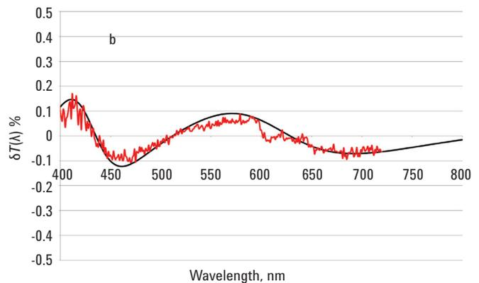
**Figure 3.** (a) Comparison of two transmittance spectra acquired using two different UMA accessories coupled to a Cary 5000 spectrophotometer. The data relates to the same  $Ta_2O_5$  sample. (b) Comparison of  $T^{(s)}(\lambda) = T^{(s,1)}(7^\circ, \lambda) - T^{(s,2)}(7^\circ, \lambda)$  calculated from experimental data (red line) and by theoretical equations (black line) [1].
