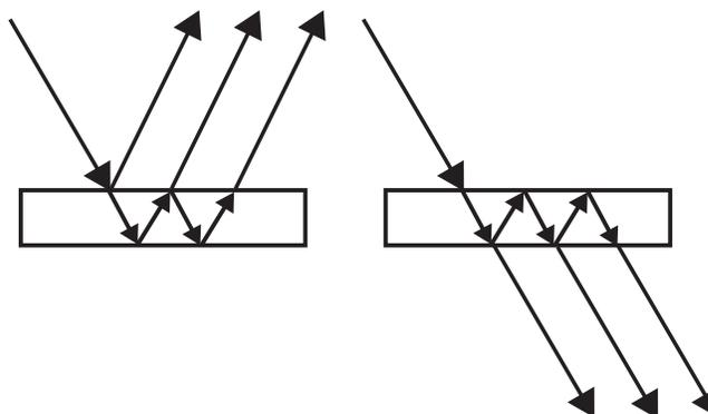
**Figure 1.** Schematic of the Agilent UMA, an absolute variable angle reflectance and transmission accessory capable of front and back surface reflection (left) and direct and inter-reflected transmission (right) measurement.
