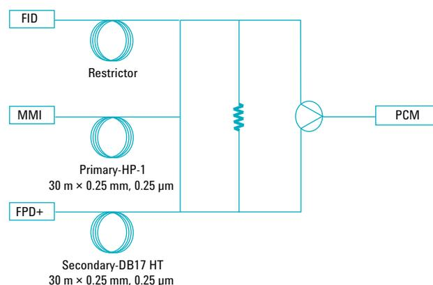
Figure 1. FPD + system with Deans switch.
