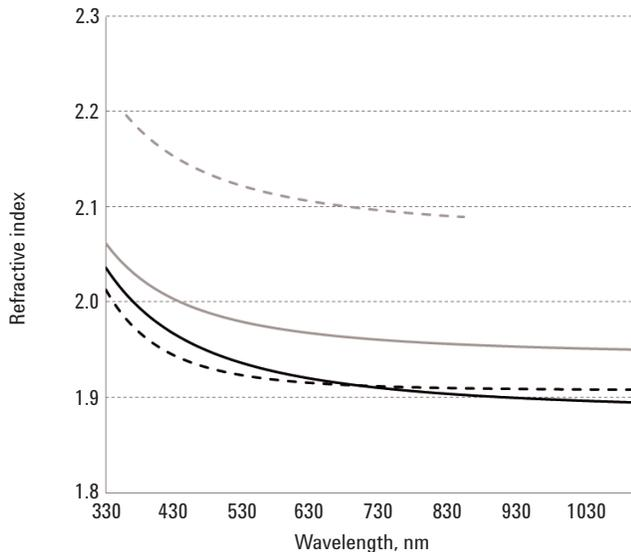
**Figure 3.** Nominal refractive index wavelength dependence of e-beam evaporated HfO<sub>2</sub> film (solid black curve), and reference refractive index wavelength dependencies of HfO<sub>2</sub> films produced by radio frequency sputtering (gray curve) and ion-beam sputtering (dashed gray curve). The dashed black curve shows the refractive index of thin HfO<sub>2</sub> film found from measurement data related to a 12-layer quarter-wave mirror.
