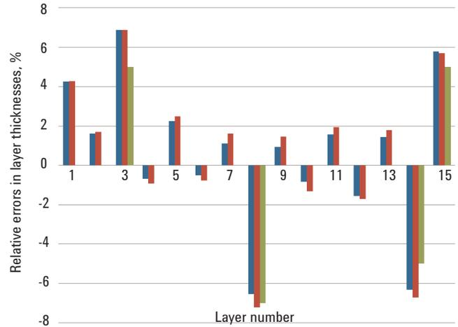
**Figure 2.** Comparison of errors in layer thicknesses of 15-layer quarter-wave mirror found on the basis of reflectance and transmittance data taken at 7°, 10°, 20°, 30°, and 40°, for the s-polarization case (blue bars) and the p-polarization case (red bars). Green bars show planned errors in the thicknesses of the third, eighth, 14th, and 15th layers.
