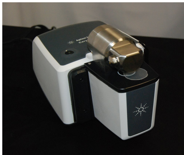
Figure 1. The Agilent DialPath transmission cell used for polymer analysis of coupons or films
