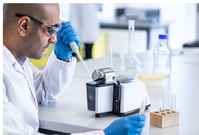
Figure 3. Agilent Cary 630 FTIR spectrometer equipped with the Agilent-exclusive DialPath sampling module. The Cary 630 is an ultra-compact, easy to use, high performance FTIR spectroscopy. Combined with DialPath technology, it is a powerful instrument for the analysis of liquids.
