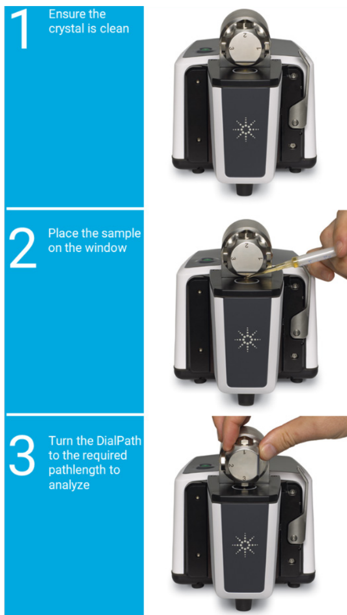
Figure 2. Liquid sample analysis. Three steps to analysis with the DialPath module.
