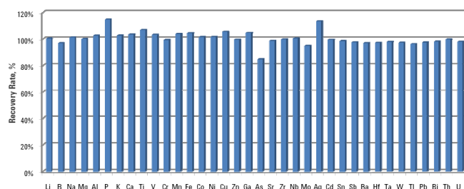
Figure 1. 5 ppb spike recovery test in TCS, confirming no loss of volatile elements during sample evaporation, and accurate recovery (between 80 and 120%) for all analytes.
