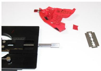
**Step 1.** Cut a small piece of sample.
