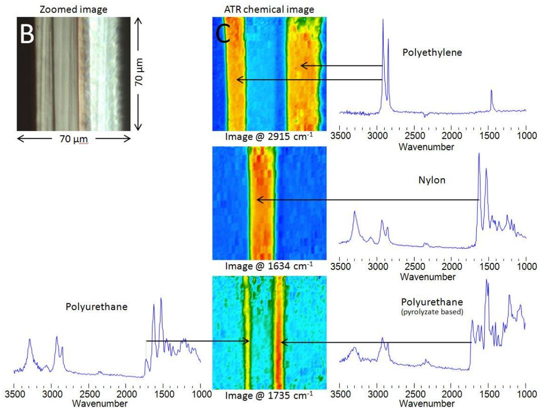
**Figure 5.** Identifying layers: B—as per Figure 4, above; and C—three chemical images created with different wavenumbers to highlight the main layers and tie layers with corresponding representative spectra as indicated by the arrows. Note: All spectra are shown in absorbance units, with axes omitted for clarity
