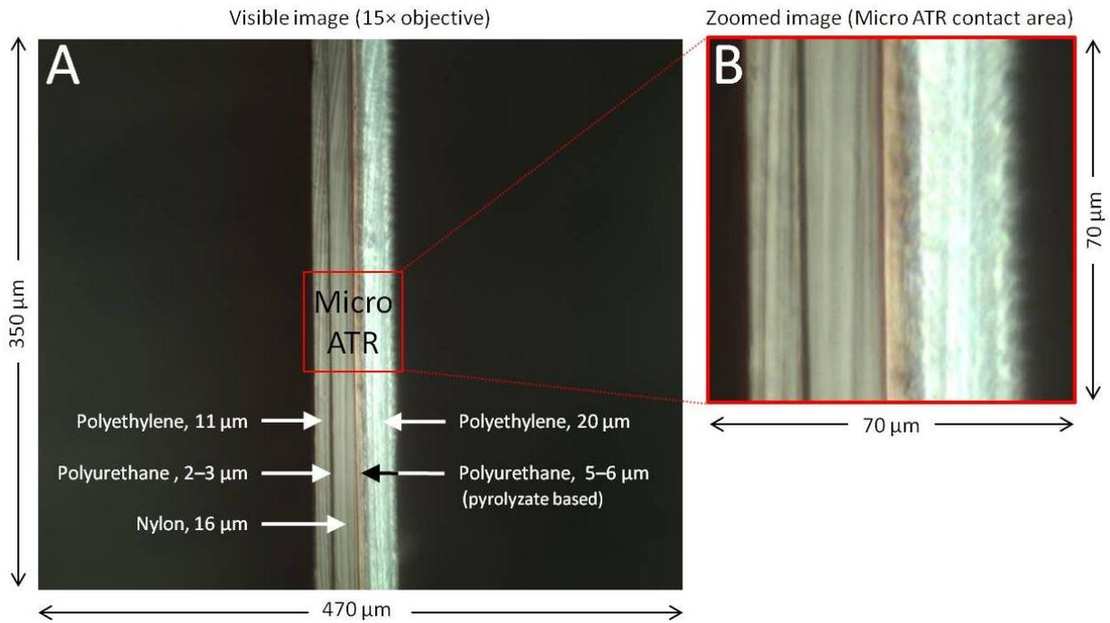
**Figure 4.** Optical images: A—the full field of view visible through microscope, annotated with the chemical composition and approximate thickness of the various layers in the sample; and B—zoomed image corresponding to the contact area of the Micro ATR
