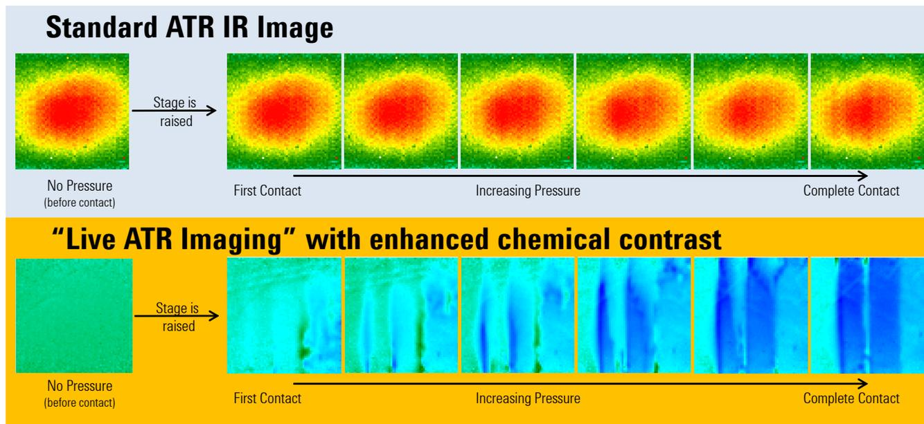
**Figure 3.** Comparison of a standard ATR IR image and Agilent’s “Live ATR imaging” with enhanced chemical contrast—clearly showing the latter can detect first contact of the ATR crystal with the sample and that contact quality can be monitored real-time as the pressure is increased and before any data collection
