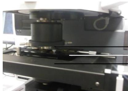
**Step 4.** Place micro-vice onto microscope stage.
