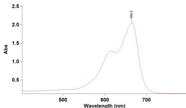
**Figure 1.** Ten superimposed wavelength scans of methylene blue (20 ppm) solution in water. As can be seen, the scans overlay perfectly confirming the accuracy of the Cary 60 UV-Vis and the absence of any photobleaching of the sample
