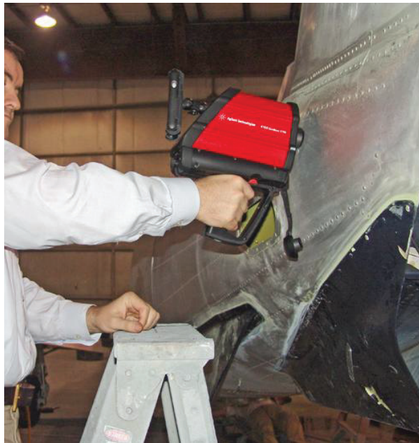
Figure 1. The handheld Agilent 4100 ExoScan FTIR with the external reflectance sample interface being used for quality inspection of an aircraft coating
