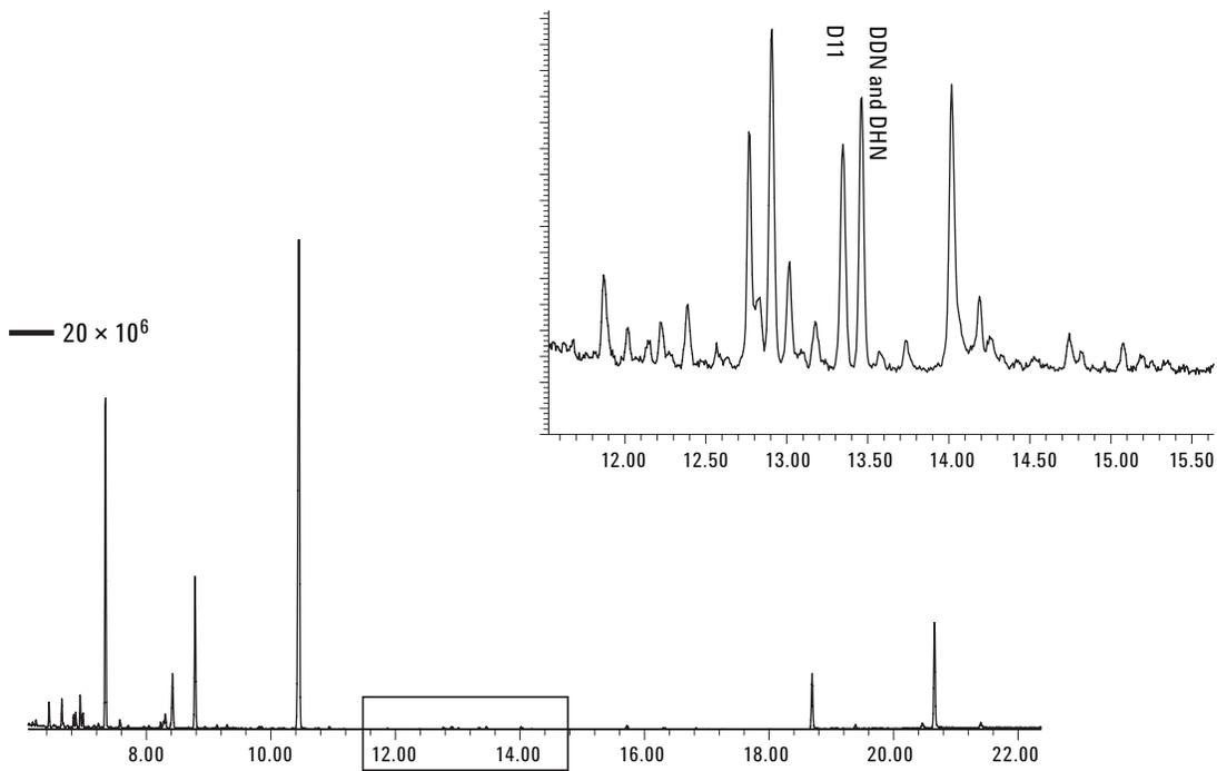
**Figure 2.** RTIC chromatogram of PCI-NH<sub>3</sub> full-scan acquisition of a typical sample. Note the intense, late-eluting (> 14 min.) components.
