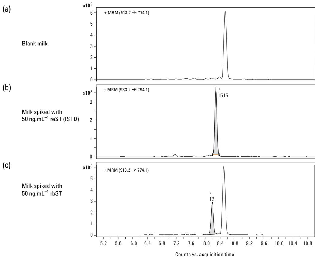
**Figure 3.** SRM ion chromatograms obtained from milk samples. The different signals correspond to (a) blank milk, (b) the same milk spiked with 50 ng.mL<sup>-1</sup> reST (internal standard), and (c) 50 ng.mL<sup>-1</sup> rbST.
