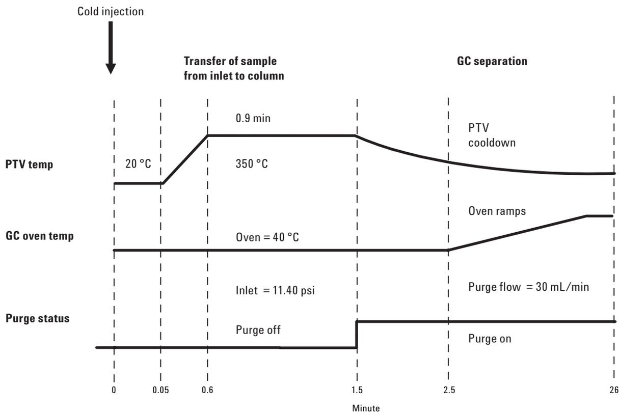
**Figure 1. PTV cold splitless temperature and flow programs.**
