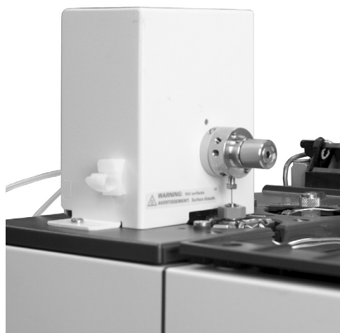
Figure 3. Agilent pneumatic air actuator/valve assembly installed on the 7890A.
