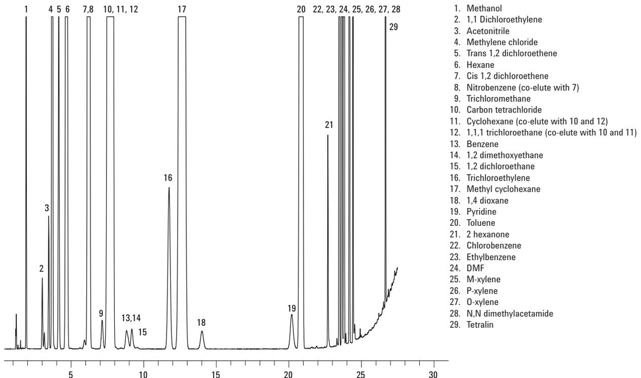
Figure 1. Class 1 and Class 2 residual solvents.
