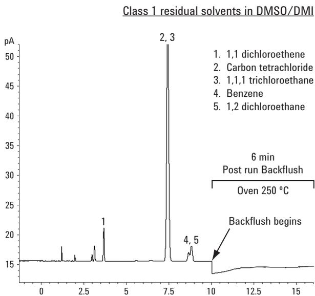
Figure 3. Backflush of Class 1 residual solvents in DMSO/DMI.
