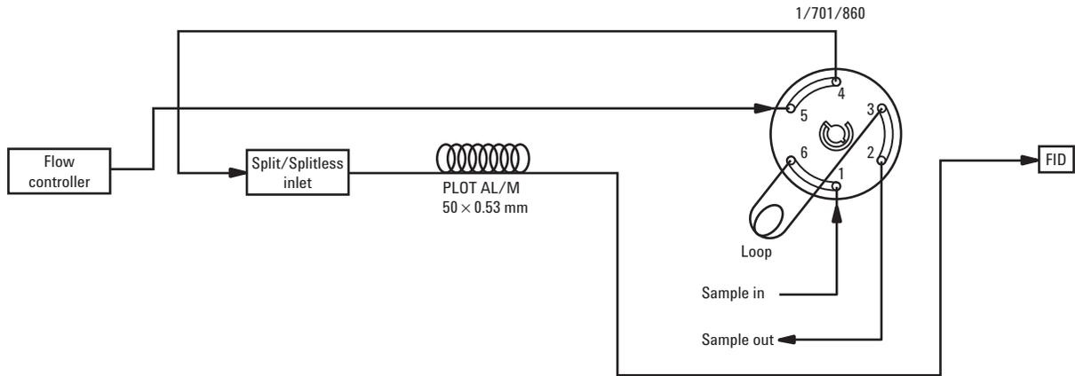
**Figure 1. System configuration.**
