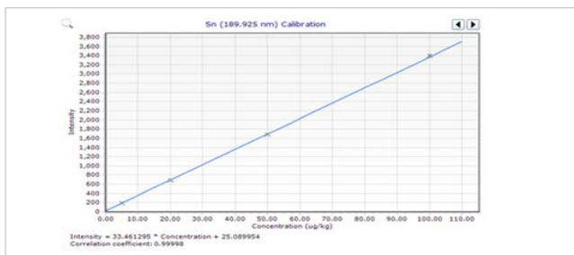
**Figure 2.** Linear calibration curves for As 193.696 nm, Hg 184.887 nm, Se 196.026 nm and Sn 189.925 nm.
