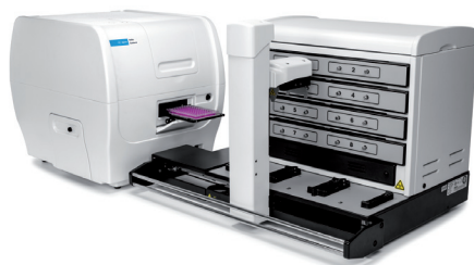
Figure 1. The Agilent BioTek BioSpa 8 automated incubator transfers microplates from the incubator to the Cytation cell imaging multimode reader.
